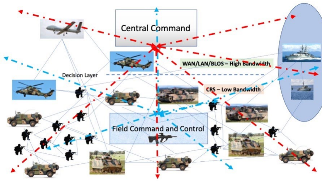
Diagram 13: Example of BMS Communication Network (Elbit System Australia)
