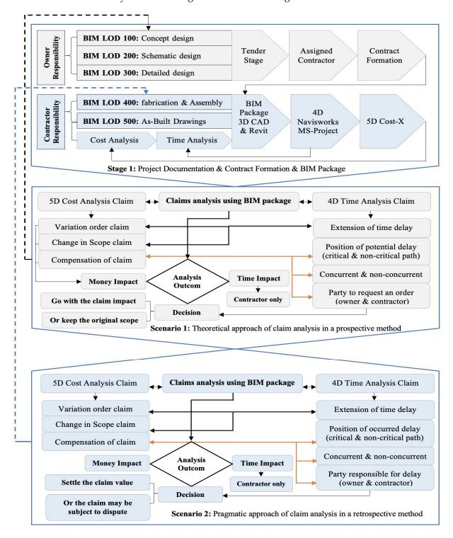
**Figure 4.** Flow chart created by the authors to show the claims analysis using the BIM package under prospective and retrospective methods.
