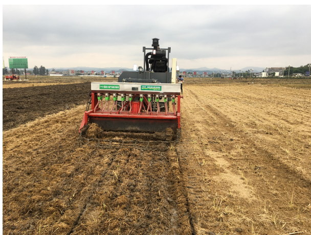
Fig. 4 – WR seeder operating in wet field with heavy rice straw retention with stainless steel chain installed behind for seed covering.
