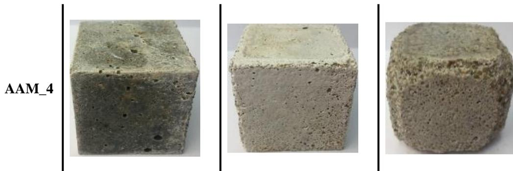
Figure 7-4. Photographs of cementing mortars after 28 days exposure to water, 3 and 5% solutions of sulphuric acid.
