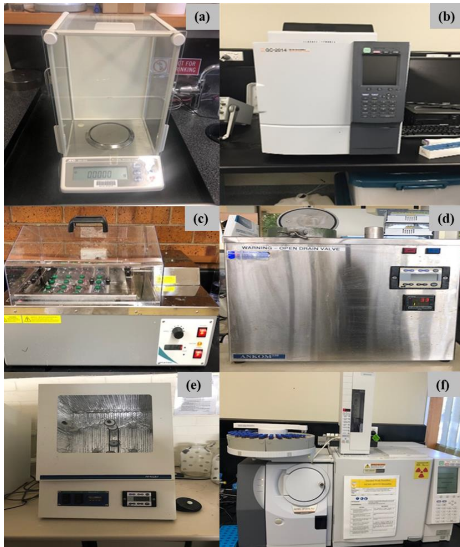
Figure 3.2: In-vitro experiment: (a) 5-digit balance, (b) multi-gas analyser (Gas Chromatograph (GC), (b) Shaking water bath, (d) fibre digestibility analyser, (e) lignin digestibility analyser and (f) spectrophotometer.
