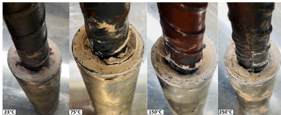
Fig. 23. Failure of pull-out specimens embedded using resin A.
