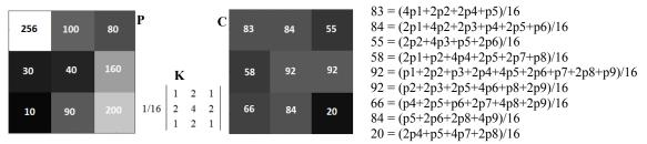
Figure 1. The original image P is multiplied (or convoluted) using a normalised kernel K. The result of the convolution is image C on the right together with the equations used to calculate image C.
