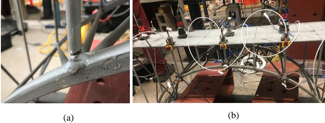
Figure 4: Column Damage on experimental model (a) damage location (b) accelerometer configuration
