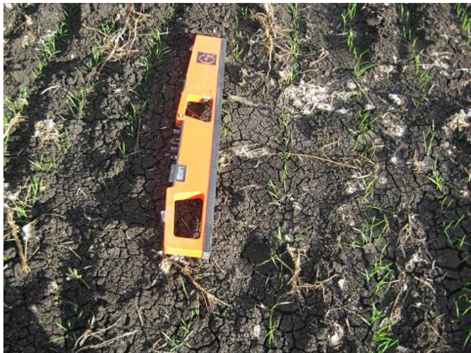
Figure 6. 1 Operation of EM38 in vertical mode (VM) at the soil surface in the field.
