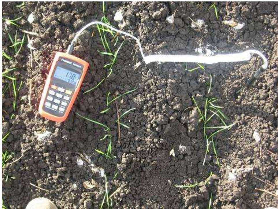
Figure 6. 3 Soil temperature measurement in the field with Omega RTD probe (meter on the left, RTD sensor on right pushed to 25 cm depth).
