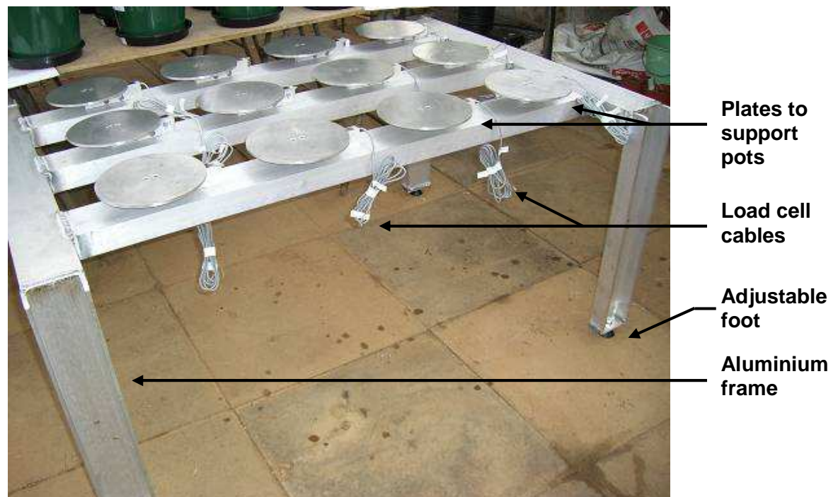
Figure 3. 1 A mini-lysimeter system consisting of an aluminium frame fitted with 12 load cells (each located under a circular aluminium plate) arranged in a 4×3 grid to represent 12 weighing lysimeters.
