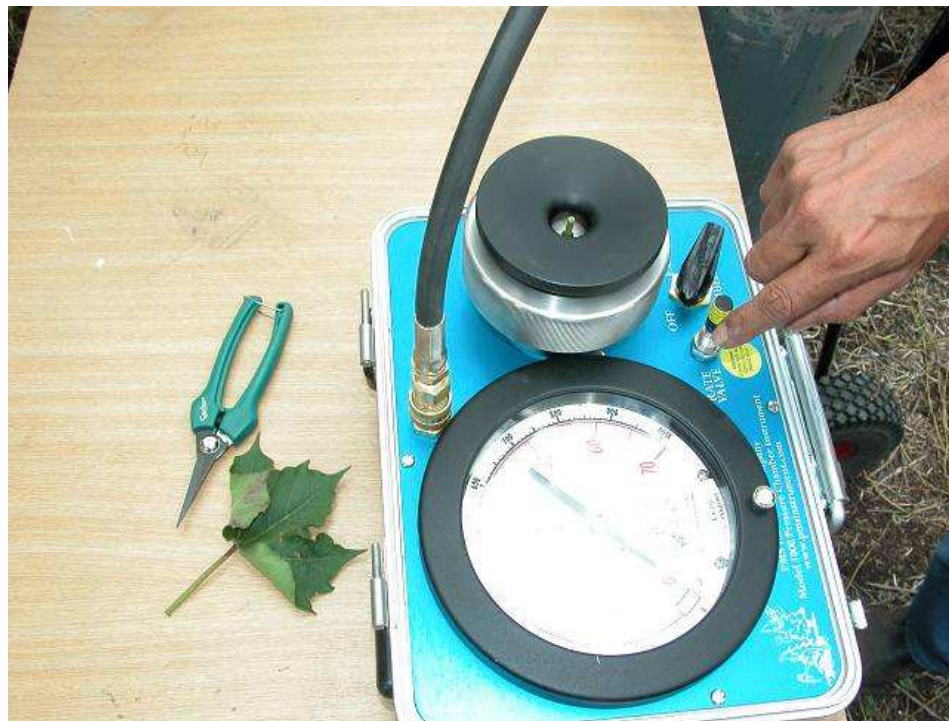
Figure 4. 5. Leaf water potential measurement for a typical cotton leaf mounted within the pressure chamber. A leaf similar to the measured leaf (not for measurement) is shown outside the pressure chamber.
