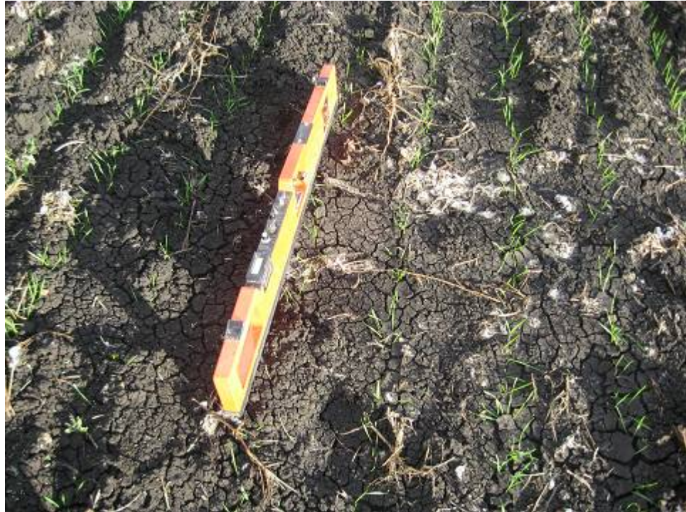
Figure 6. 1 Operation of EM38 in vertical mode (VM) at the soil surface in the field.
