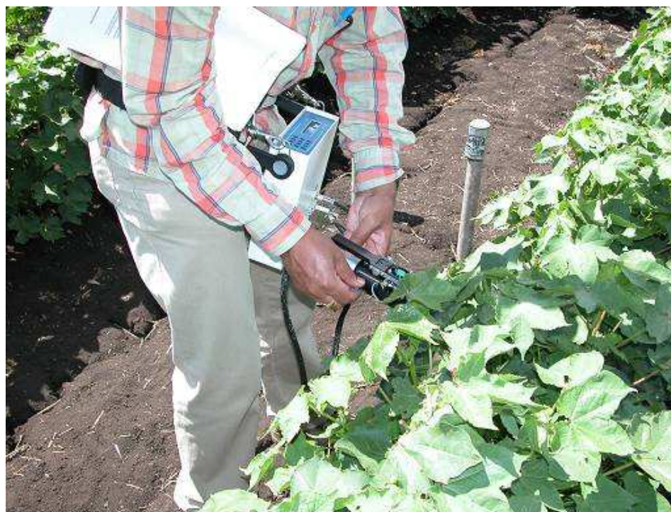
Figure 4.6. Stomatal conductance measurement for a typical cotton leaf with PMR-5 steady-state porometer.
