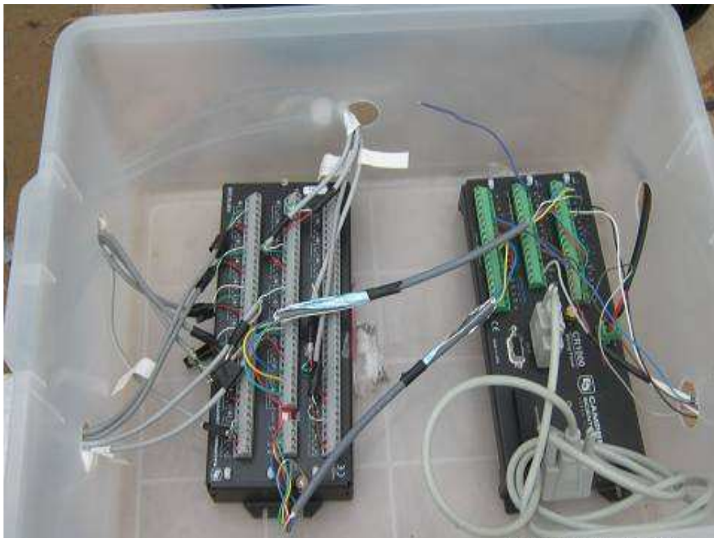
Figure 3. 4 The connections between relay multiplexer (on left) with the data logger (on right) shown for the mini-lysimeter system.
