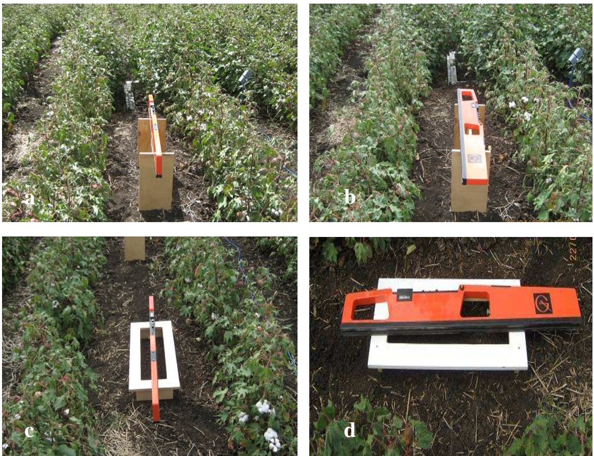
Figure 6. 5 EM38 measurements in the field at various heights above the ground shown for a cotton field. (a) VM – 0.4 m height, (b) HM – 0.4 m, (c) VM – 0.1 m and (d) HM – 0.1 m.
