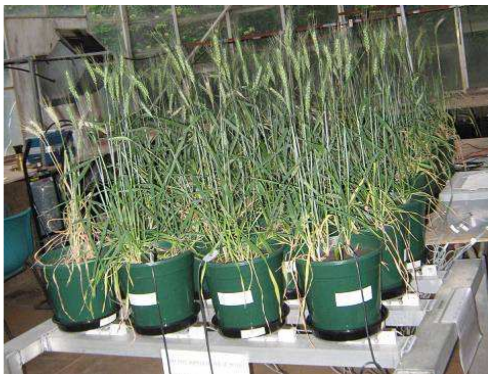
Figure 5. 2 Wheat growing in pots in the glasshouse experiment. Front three rows of pots are placed over the mini-lysimeter system.
