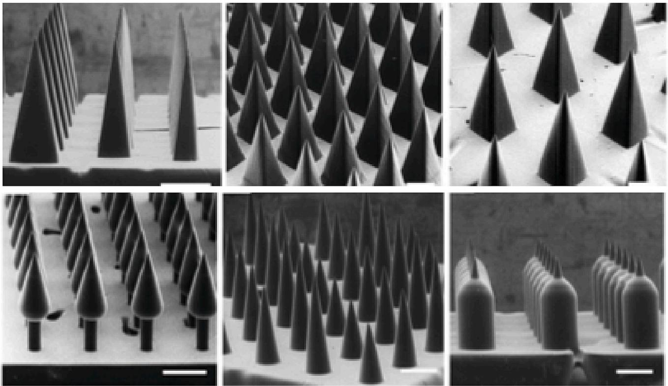
Fig. 3. Different geometries of MN tip (cylindrical, rectangular, pyramidal, conical, octagonal and quadrangular). Reprinted with permission from (Nagarkar et al., 2020). Copyright 2020, Elsevier.
