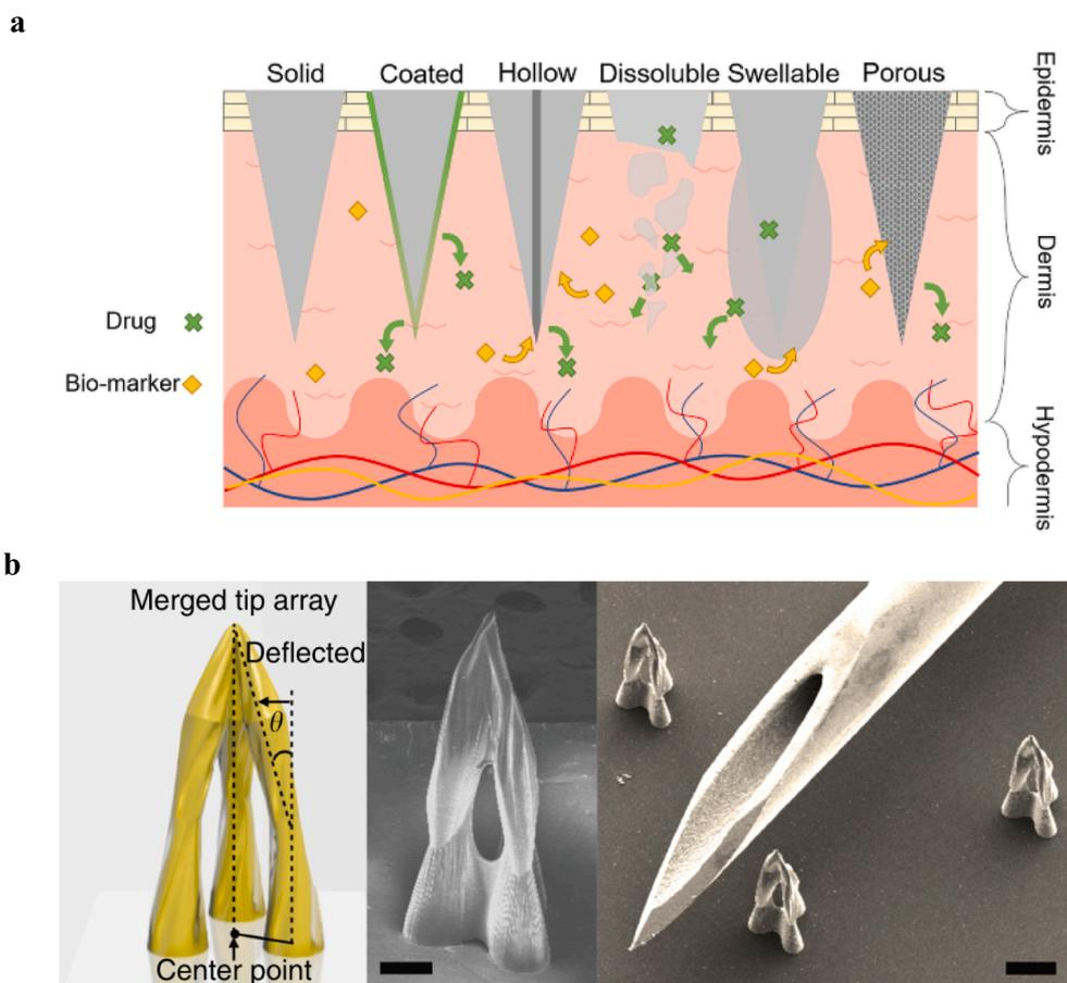
**Fig. 1.** Different types of MNs: (a) solid, coated, hollow, dissolvable, swellable, and porous MNs. Reprinted with permission from (Bao et al., 2022). Reproduced under the terms of the CC-BY 4.0 license. Copyright 2021, Springer Nature. (b) Merged-tip MNs compared with a conventional steel hypodermic needle. Adapted with permission from (Lim et al., 2018). Reproduced under the terms of the CC-BY 4.0 license. Copyright 2018, Springer Nature.
