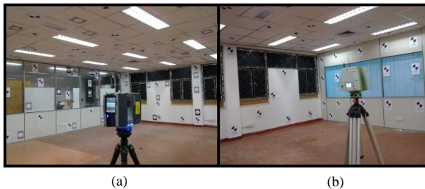
Figure 2 Self-calibration of the panoramic (a) and hybrid scanners (b).
