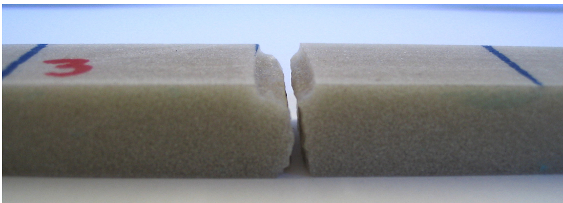
Figure 5.12 A flexure specimen with a 10% filler content showing the reduced size of the break away segment from the compression face.
