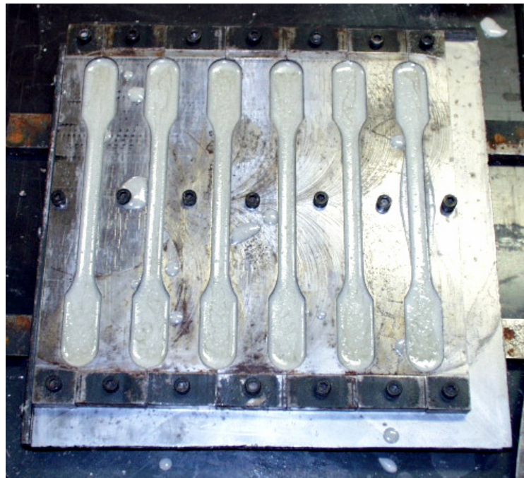
Figure 5.2 Tensile test specimens cast in a multiple cavity “dog-bone” shaped mould.
