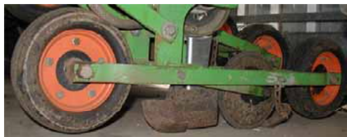
Figure 103: A seed-firming wheel following a runner type furrow opener
