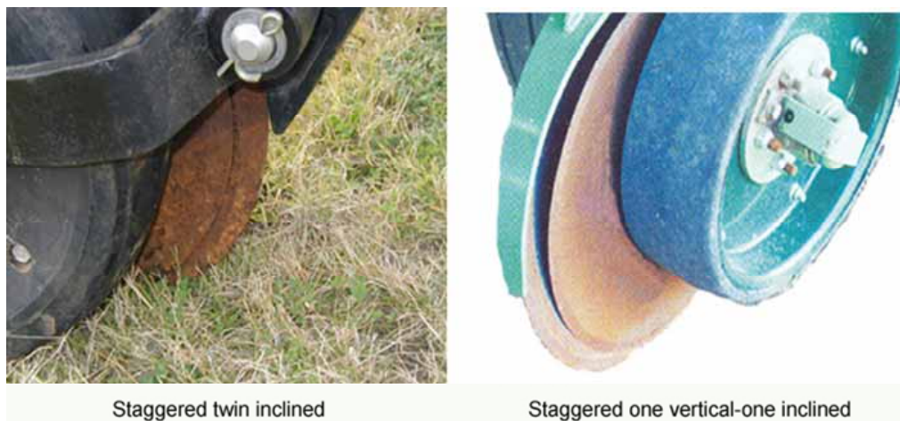
Figure 75: Staggered 'twin inclined' and 'one vertical-one inclined' types of double disc opener
