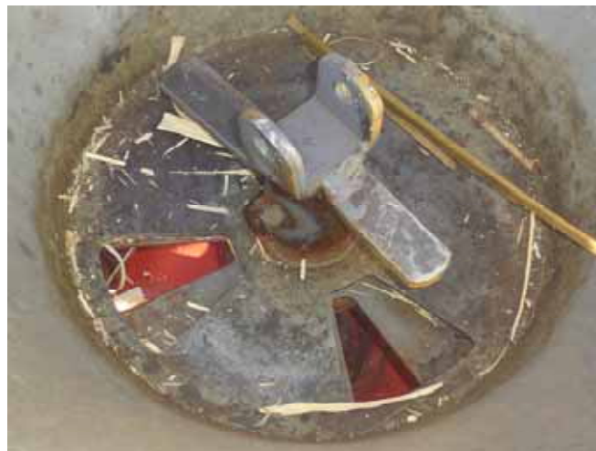
Figure 164: A stationary opening type seed meter using a sliding plate to adjust the outlet size
