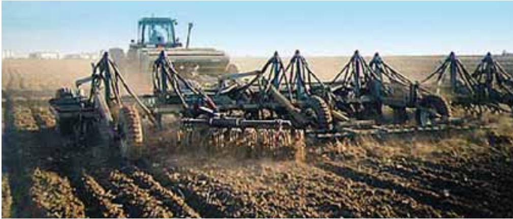
Figure 138: Coil press unit used as non row specific seedbed levelling device
