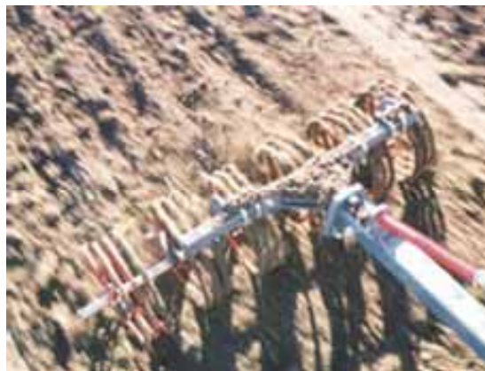
Figure 137: Press coil unit in operation
