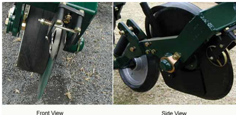
Figure 64: The front and side views of a single compound angled disc coulters type furrow opener
