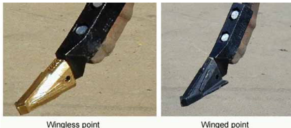
Figure 84: Winged and wingless versions of the same basic opener shape
