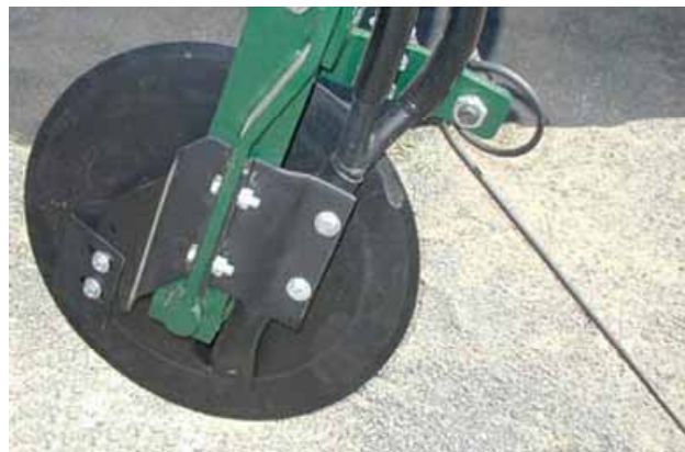
Figure 120: A single finger type covering device
