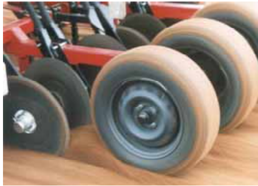
Figure 68: Opposed single disc coulters sharing a common press wheel
