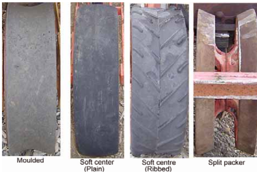
Figure 128: Zero pressure press wheel types
