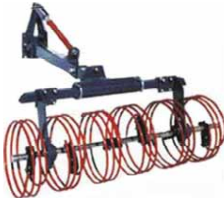
Figure 136: A gang of coil press seedbed firming devices
