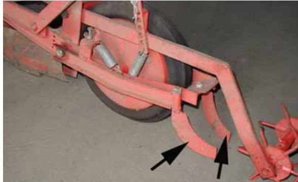
Figure 114: Opposed knife type covering devices
