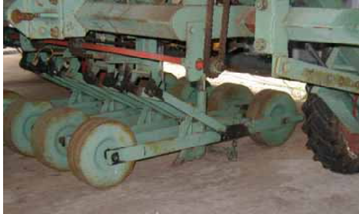
Figure 162: A twin wheel type of the trailing arm system of depth control
