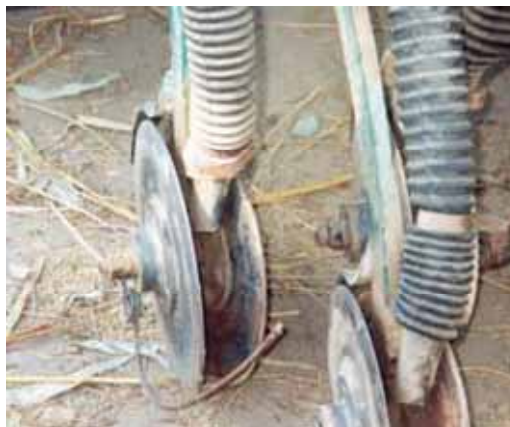
Figure 77: Seed placement via a dropper tube terminating well above the furrow base
