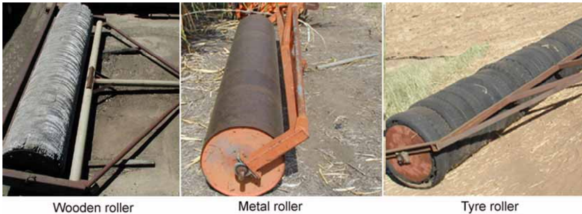
Figure 141: Examples of roller types
