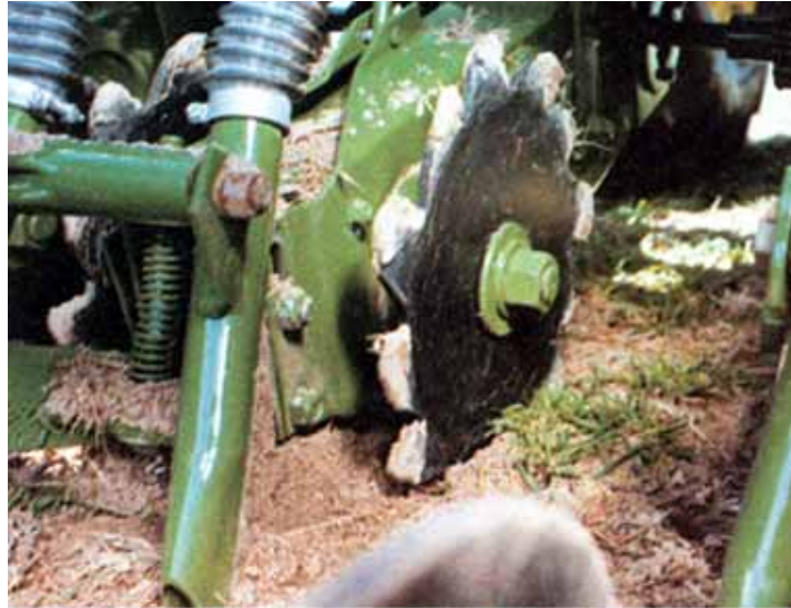
Figure 99: The rear side view of a powered type furrow opener
