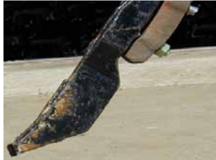
Figure 87: A typical knife type tine opener
