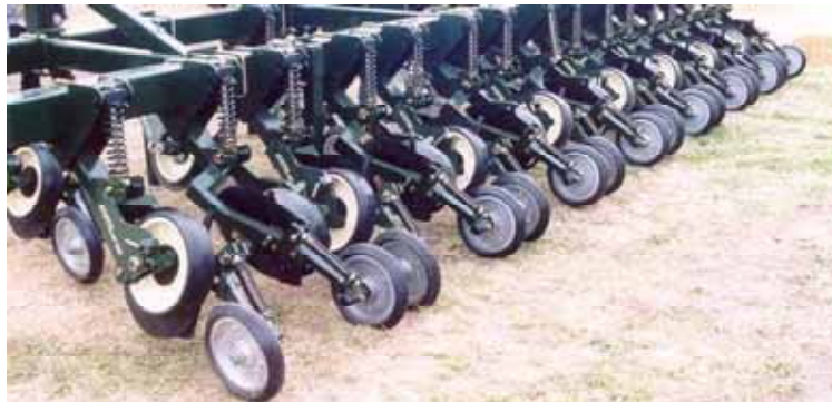
Figure 66: Openers arranged in opposed pairs across the full width of the machine
