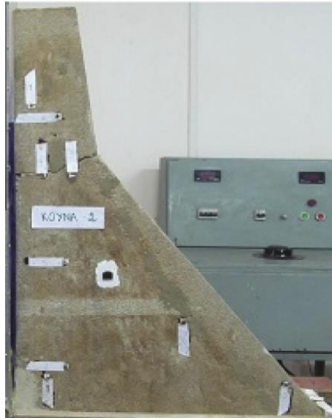
Figure 7. Experimental simulation of cracks under on a Koyna dam model [26]
