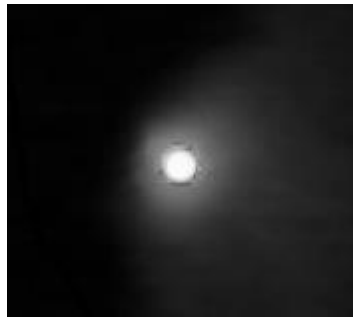
Figure 20: A grayscale image of the sun, taken with a 340 nm filter covered Samsung Galaxy 5 smartphone camera (magnified image). (Igoe et al. 2013b).
