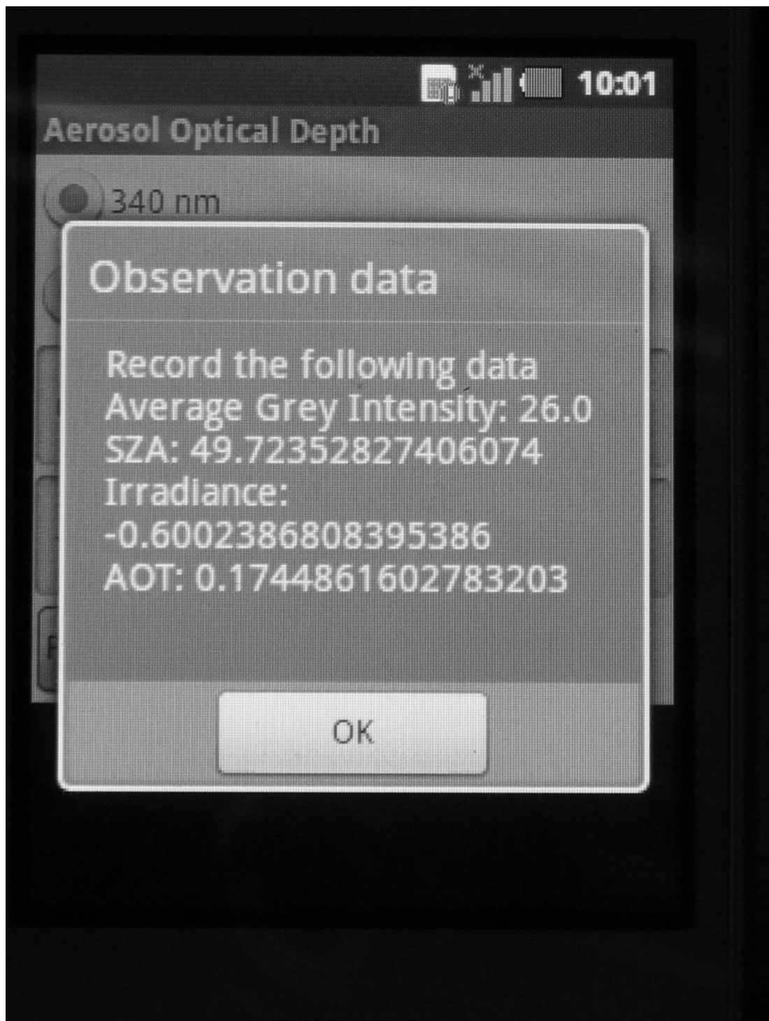
Figure 42: Raw data dialog box as the final stage of the Android app calculations (note, the irradiance value is actually its natural log). The apparent precision in the data is due to the simplicity in the app code.
