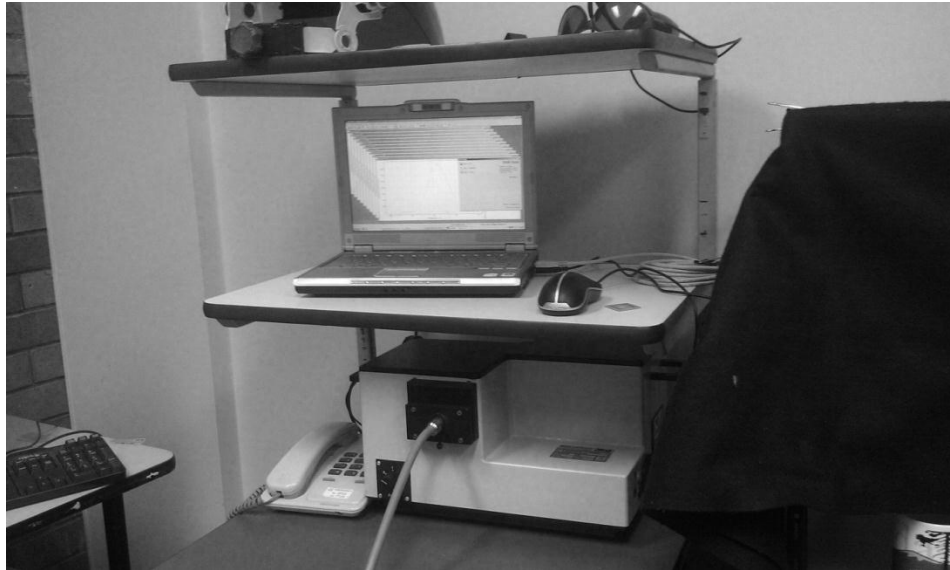
Figure 11: Spectroradiometer used for the irradiance measurements in the feasibility tests.
