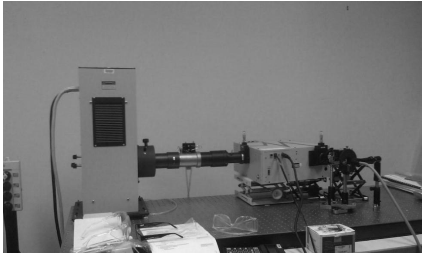
Figure 10: Irradiation monochromator used for producing a stable beam of approximately 10 nm FWHM for the feasibility studies.
