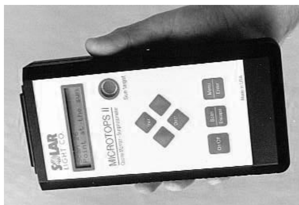
Figure 12: Microtops II Model 540 sunphotometer, used in field calibration tests for measuring direct UV and AOD (Image by Solar Light).
