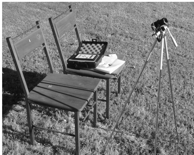
Figure 19: Field setup, including smartphone with filters on top of the tripod. The Microtops sunphotometer pictured was used to calibrate the smartphone camera's image sensor data.
