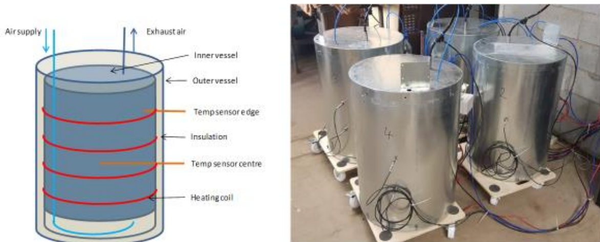
Figure 10 Schematic and actual view of small-scale composting reactors
