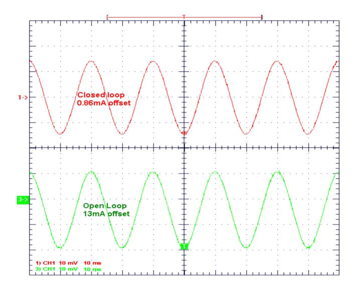
Figure 7: DC Offset sensor output
