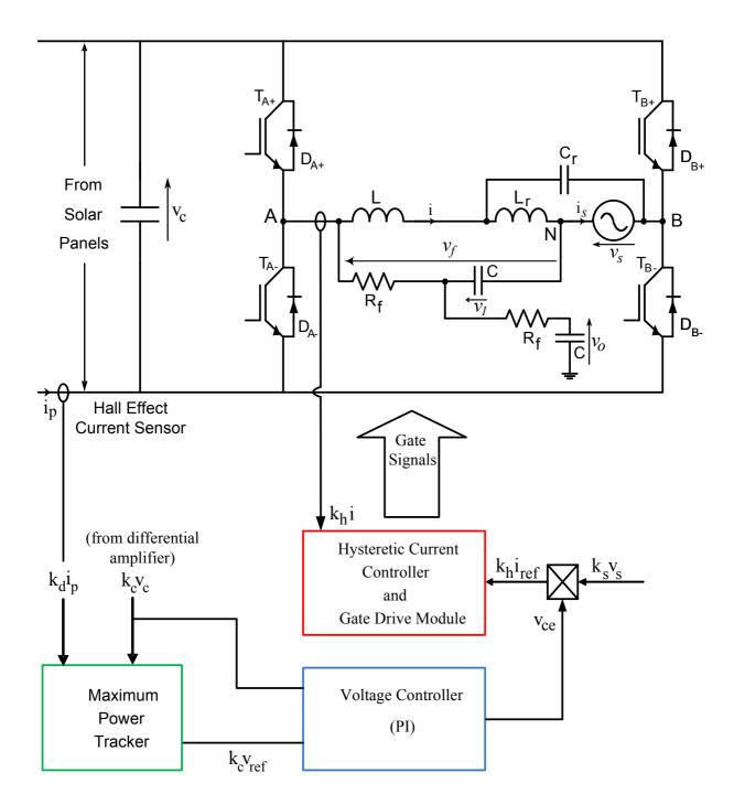
$k_{c},\,k_{d},\!k_{h}$  and  $k_{s}$  are current or voltage sensor constants
