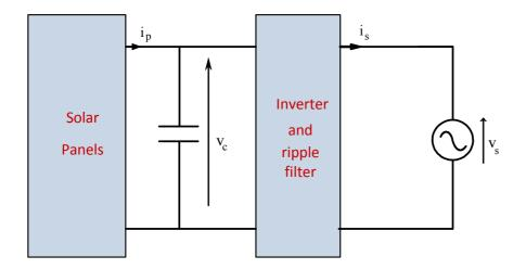
Figure 1: Grid-Connected PV System
