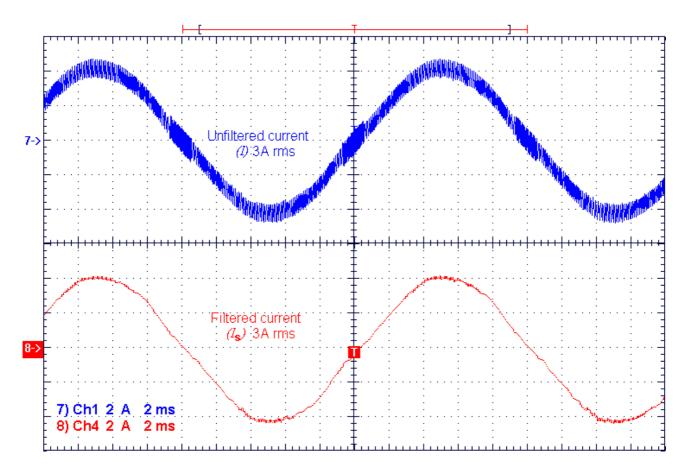
Figure 3: Inverter Output Current Waveform ( $I_{ref} = 3A$ )
