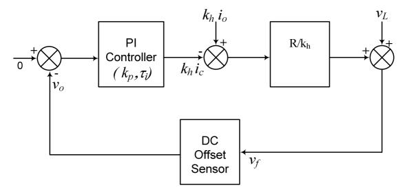
Figure 4: DC offset sensor block diagram
