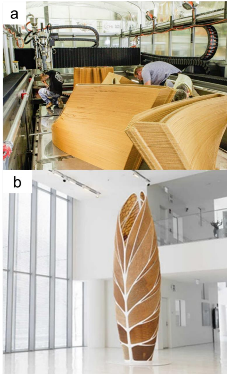
Figure 2-14 (a) 3D printing pavilions by researchers at Oak Ridge National Laboratory used a bamboo biocomposite material (Photo Credit: Oak Ridge National Laboratory) [93] and (b) installation Aguahoja I created by Neri Oxman and the Mediated Matter group with cellulose, chitosan, and pectin (Source: Mediated Matter Group) [93].
