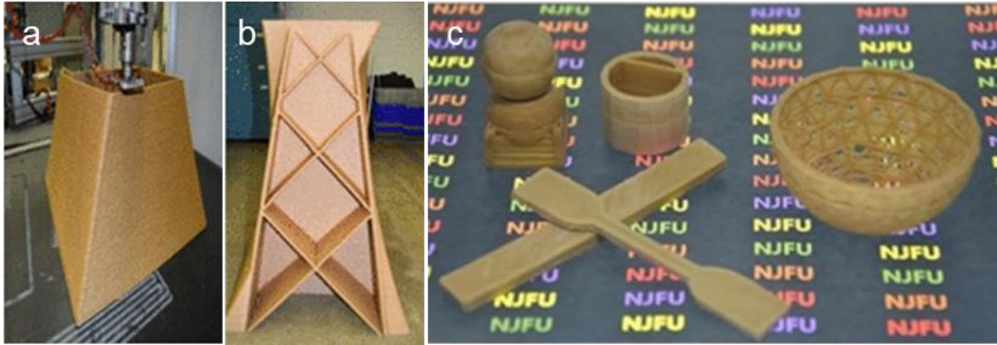
Figure 2-15 (a) Large-scale 3D printing process and (b) a completed 3D-printed podium base using poplar/PLA composite [66], and (c) the FDM printed products with PLA/30% MNC composite [11].
