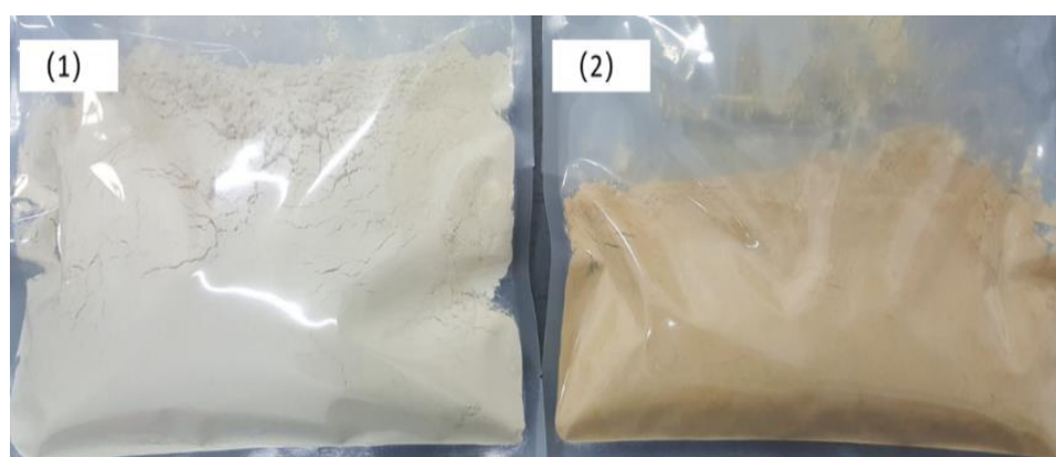
Figure 5-6 Digital photos of (1) HH and (2) BP with the same weight showing the difference in bulk density between HH and BP.
