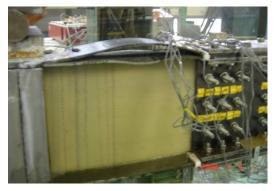
Figure 13. Failure mode of hybrid FRP girder with bolted and epoxy bonded joints
