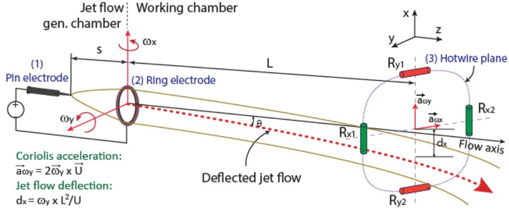
Fig. 2. Principle of the ion wind gyroscope.
