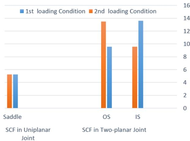
**Fig. 11.** Comparing the uniplanar and two-planar SCF values under the 1<sup>st</sup> and 2<sup>nd</sup> OPB moment loading conditions
