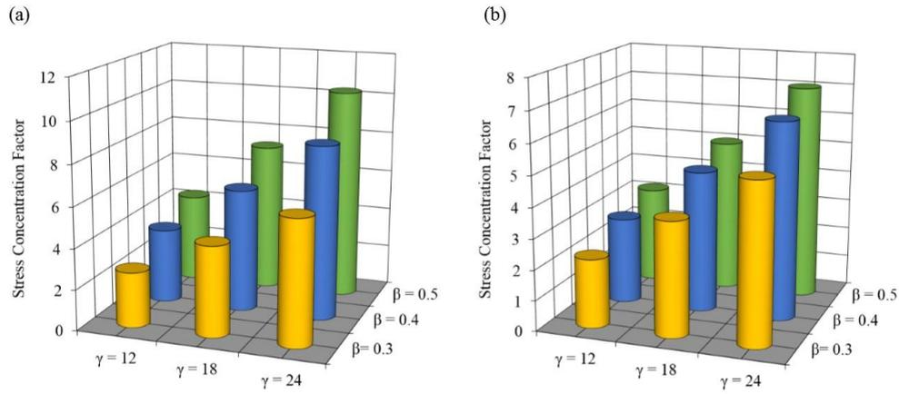
**Fig. 9.** The effect of the  $\gamma$  on the SCFs at different positions ( $\alpha = 16$ ,  $\tau = 0.7$ ; 1<sup>st</sup> OPB moment loading condition): (a) Inner saddle, (b) Outer saddle
