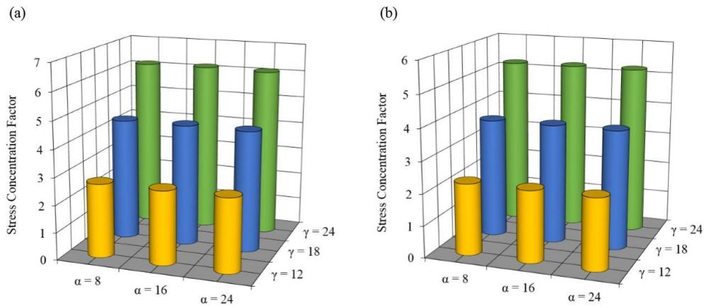
**Fig. 10.** The effect of the  $\alpha$  on the SCFs at different positions ( $\beta = 0.4$ ,  $\tau = 0.7$ , 1<sup>st</sup> OPB moment loading condition): (a) Inner saddle, (b) Outer saddle
