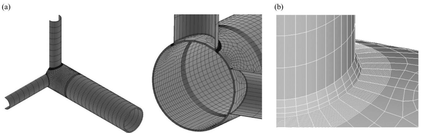
**Fig. 4.** Generated mesh by the sub-zone scheme: (a) Half of the joint under the OPB moment loading condition, (b) Regions adjacent to the brace-to-chord intersection
