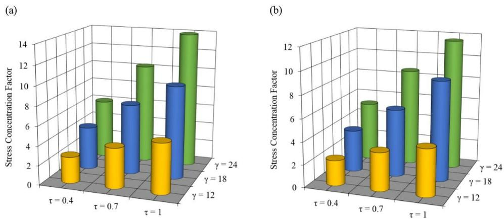
**Fig. 7.** The effect of the  $\tau$  on the SCFs at different positions ( $\beta = 0.4$ ,  $\alpha = 16$ ; 1<sup>st</sup> OPB moment loading condition): (a) Inner saddle, (b) Outer saddle
