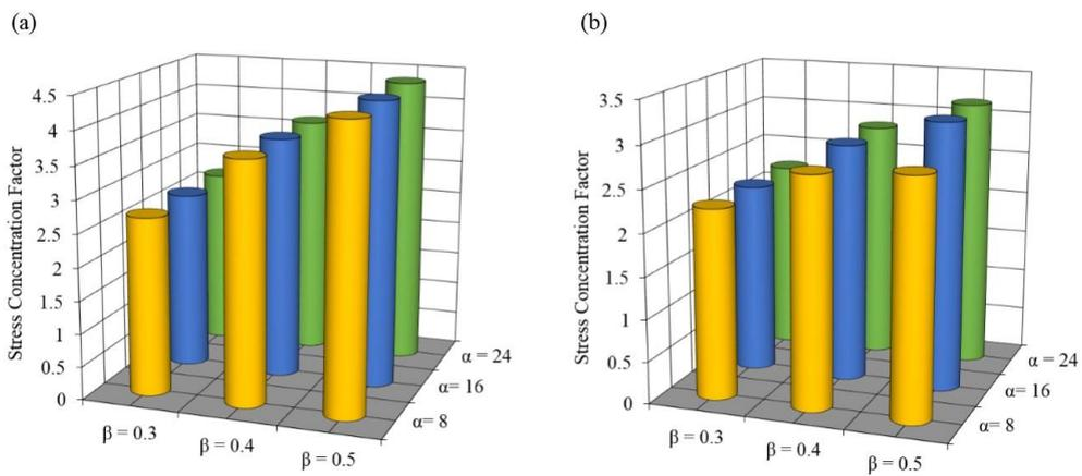
**Fig. 8.** The effect of the  $\beta$  on the SCFs at different positions ( $\tau = 0.7$ ,  $\gamma = 18$ ; 1<sup>st</sup> OPB moment loading condition): (a) Inner saddle, (b) Outer saddle
