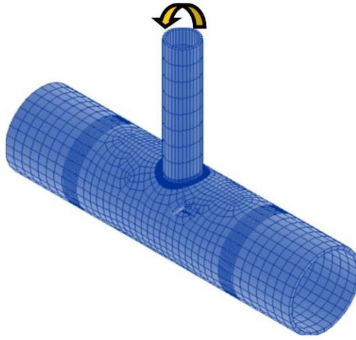
**Fig. 6.** Validating FE model generated for the comparison of the results with HSE OTH 354 [5] experimental measurements
