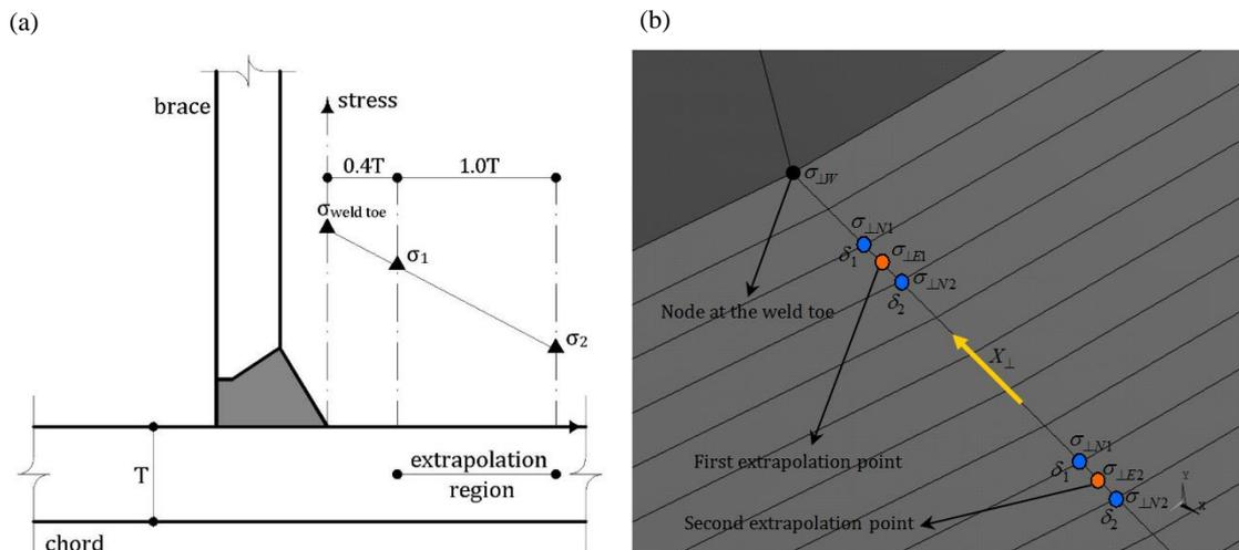
**Fig. 5.** (a) Extrapolation method according to IIW XV-E [66], (b) Required interpolations and extrapolations to extract the HSS value at the weld toe
