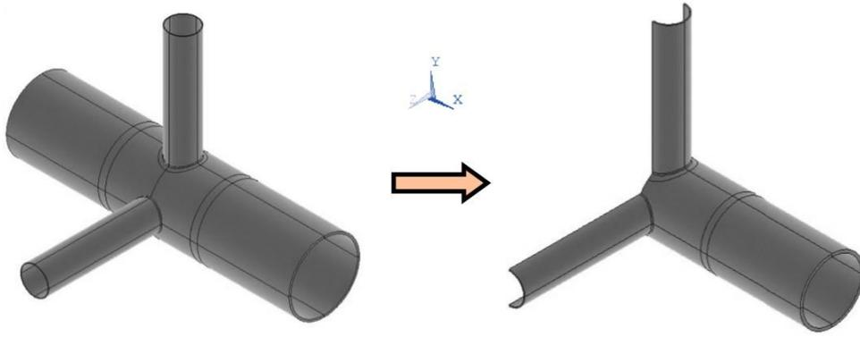
**Fig. 3.** One quarter of the entire two-planar TT-joint that is required to be modeled under studied OPB moment loading conditions
