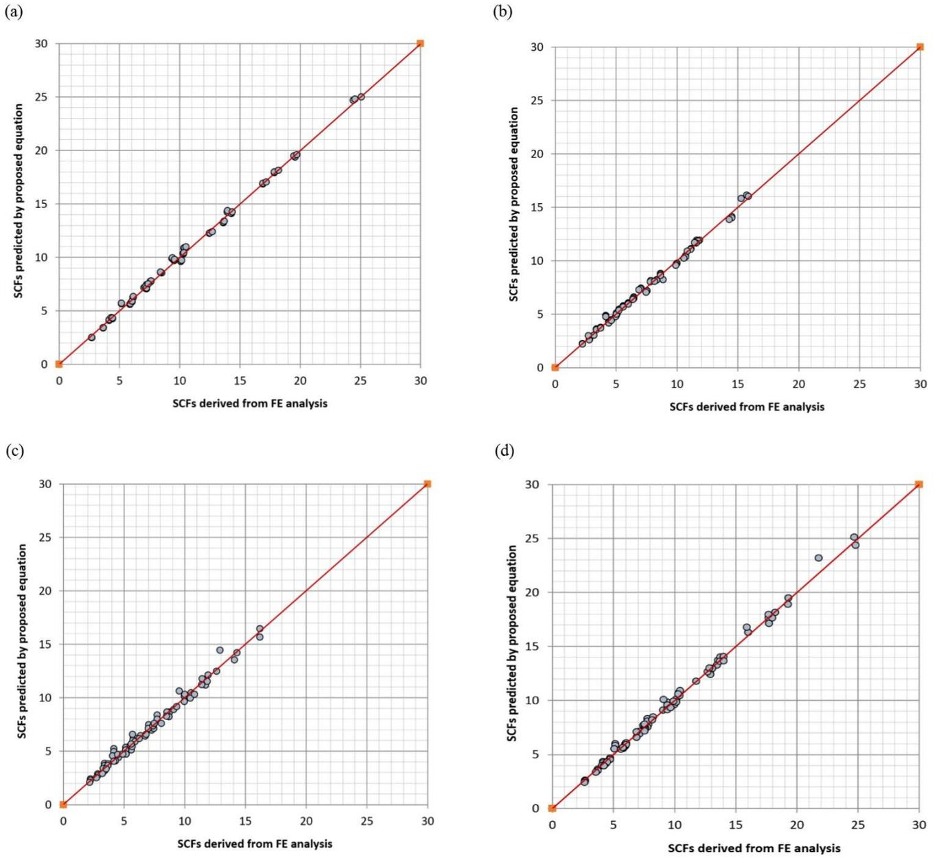
**Fig. 12.** Comparison of 81 SCF values calculated by the proposed equations with the corresponding SCFs extracted from the FE analysis: (a) Eq. (13), (b) Eq. (14), (c) Eq. (15), (d) Eq. (16)
