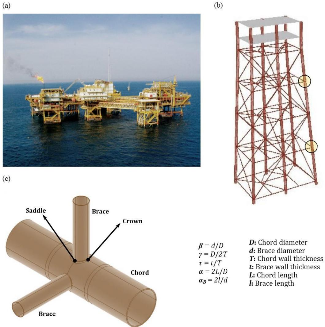
**Fig. 1.** (a) Jacket-type offshore platforms during service, (b) Two-planar tubular DT-joints in a jacket structure, (c) Geometrical notation for a multi-planar tubular TT-joint
