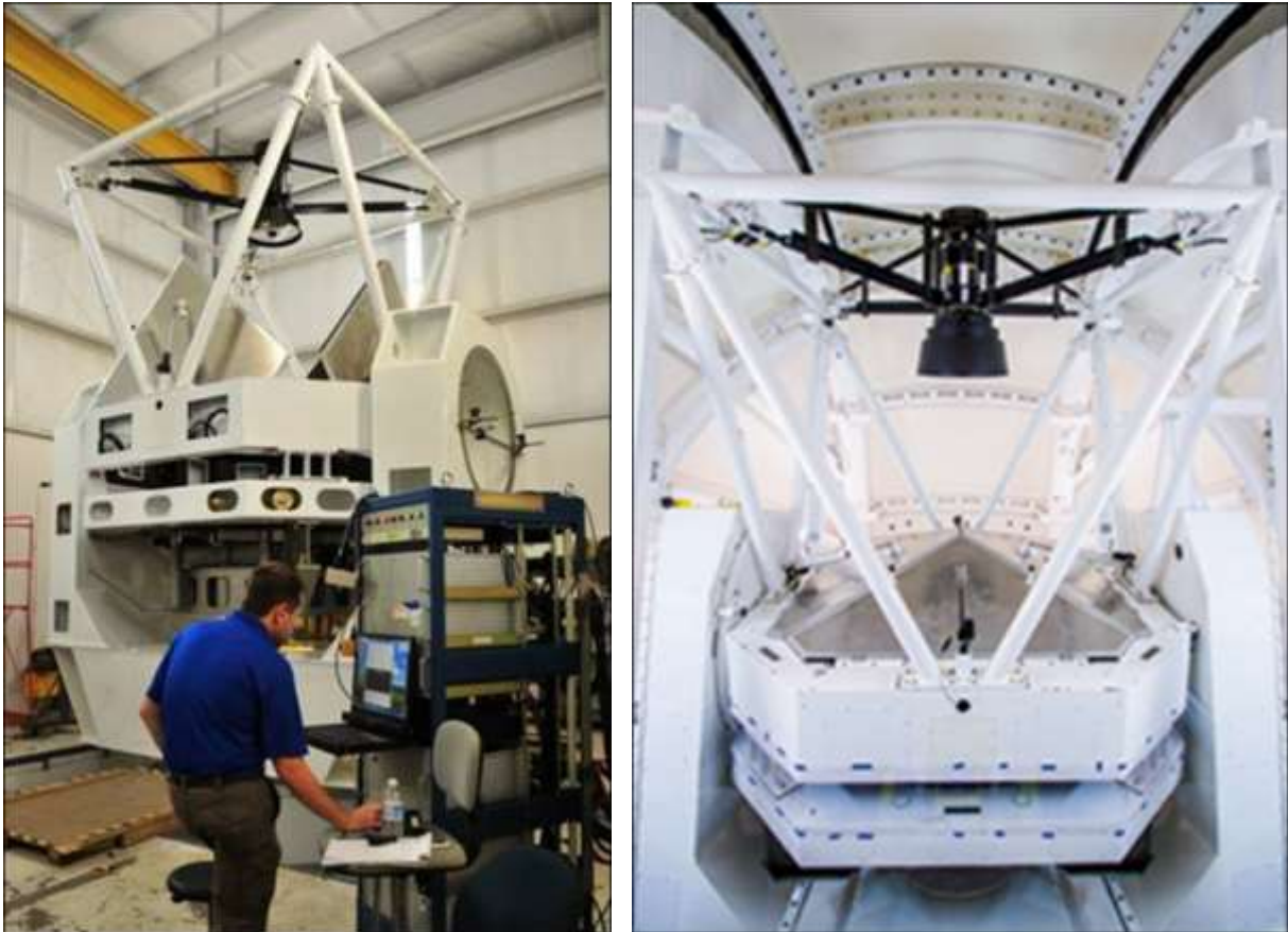
Figure 30: Two views of the automated 2.4-m Ritchey-Chrétien Thai National Telescope (TNT). Left: undergoing testing prior to its installation at the TNO; right: installed and operational at the TNO (courtesy: NARIT).
