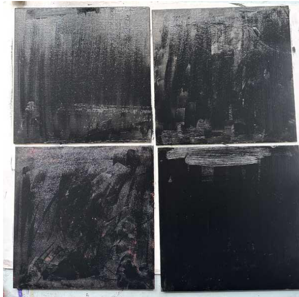
Figure 131: First coat of bitumen paint on canvas applied with a brush
