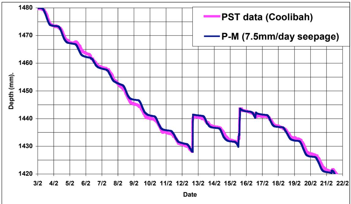
Figure 6 Graph of PST derived water depth data (thick pink line) with two instances where there was inflow of water to the dam from rainfall. Superimposed on the PST trace is a prediction of evaporation produced by EvapCalc software (thin black line) based upon Penman-Monteith (P-M) theory with a Morton based advection correction for the dry to wet transition.
