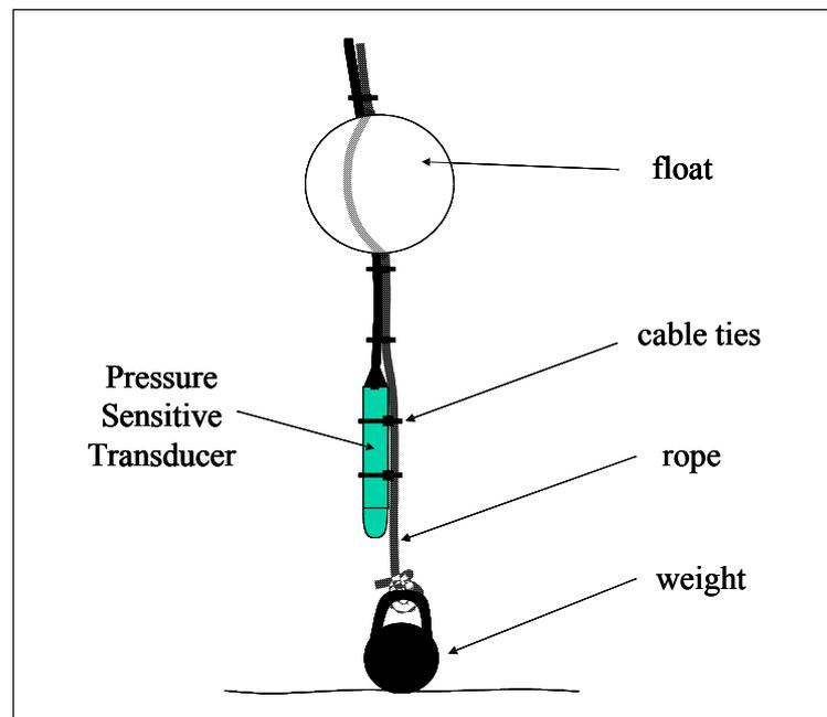
Figure 1 The PST water depth sensor suspension mechanism (schematic).
