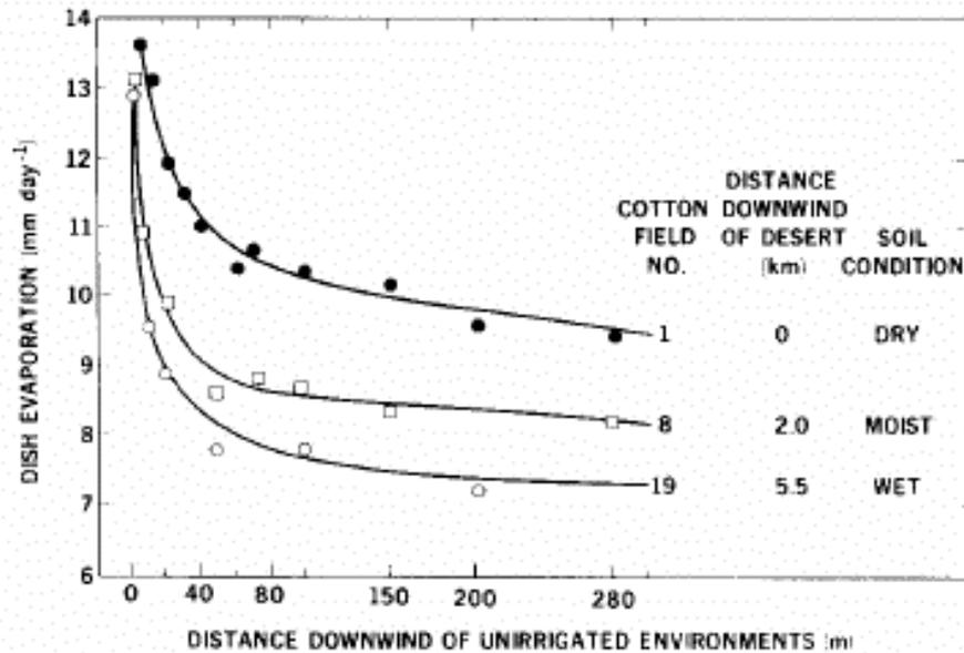
Figure 2 Davenport and Hudson (1967) comparison of evaporation rates (measured using 113mm x 36mm dishes) across irrigated cotton fields on December 27th, 1963
