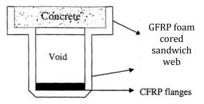
Figure 7. Hybrid box beam concept [18].
