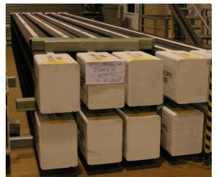
Figure 9. Glue-laminated sandwich bridge girder.
