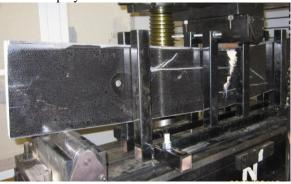
Figure 14. Flexural test of a sandwich waler
