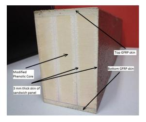
Figure 15. Hybrid glulam composite sandwich beam
