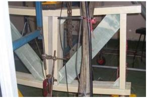
Figure 10. Modular composite truss panel [22].
