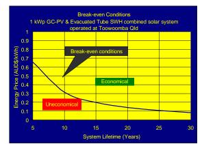
**Figure 5.** Break-even conditions of the 1 kW GC-PV operating alongside a 1.37m<sup>2</sup>/120 Litre evacuated tube SWH system.
