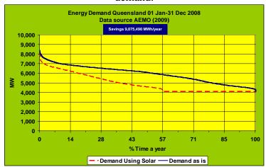
Figure 10 Solar energy contributing fully covering diurnal electrical peak demand in Queensland.
