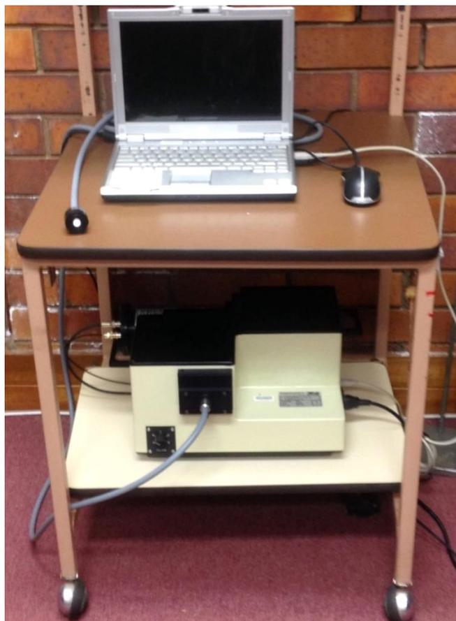
**Figure 2.10** Portable scanning spectroradiometer used for irradiance measurements in the laboratory.
