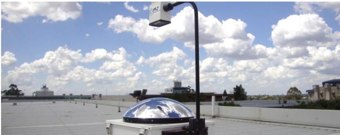
**Figure 2.4** Total Sky Imager used to record cloud cover (USQ 2016).
