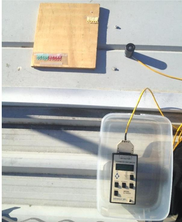
**Figure 2.6** IL1400 broadband meter recording UVB exposure.
