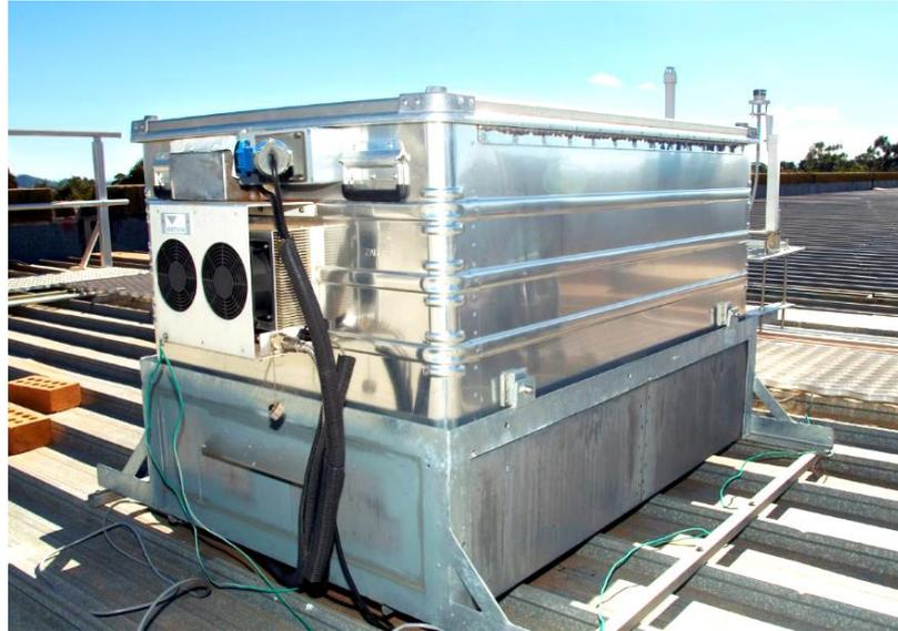
**Figure 2.3** Bentham spectroradiometer in the Envirobox (Schouten 2009).
