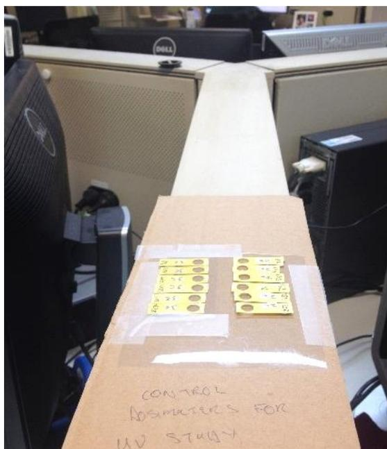
**Figure 5.4** Control dosimeters in position indoors at site 1, UVA dosimeters are on the left and PPO dosimeters are on the right.
