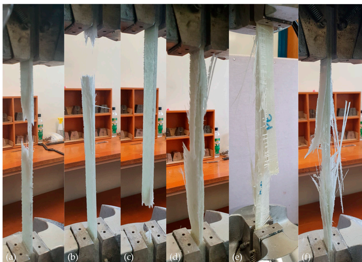
Figure 3. Failure of the specimens recorded during the test. (a) Lateral failure at the middle of the gauge, (b) lateral failure at the top tab, (c) lateral failure at the bottom tab, (d) edge delamination at the middle of the gauge, (e) surface delamination at the middle of the gauge, and (f) explosive failure at the middle of the gauge.
