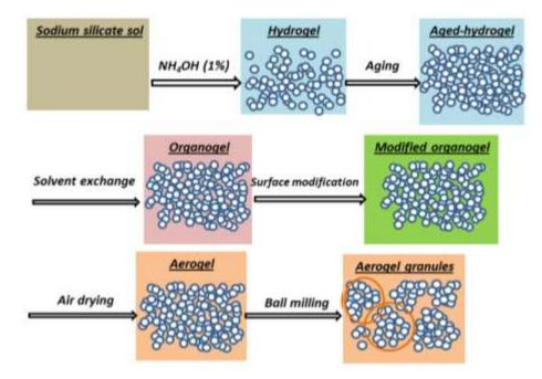
Figure. 1 A schematic of aerogel synthesis.
