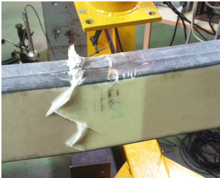
Figure 7.27 Beam Failure Due to Collapse of Compressive Reinforcement
