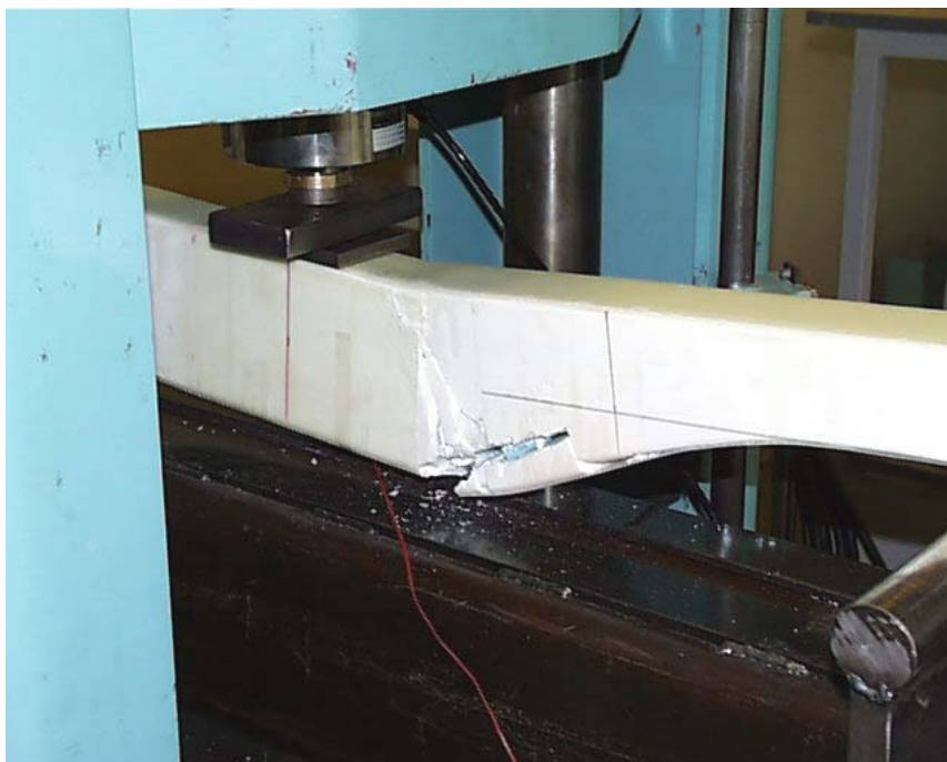
Figure D.14 (b) Failure of Neck Section #5
