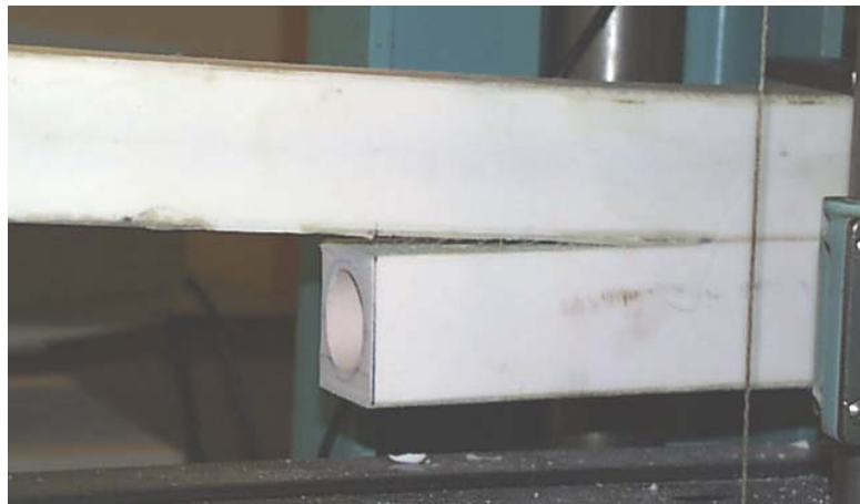
Figure 7.19 Failure of Neck Section #1
