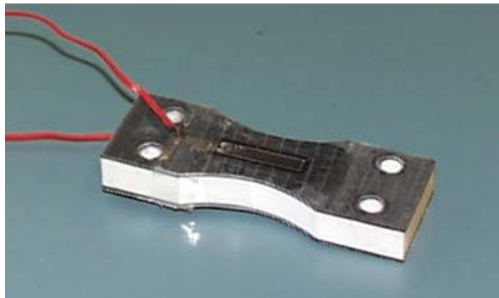
Figure G.5 Fatigue Specimen with PU Elastomer Core
