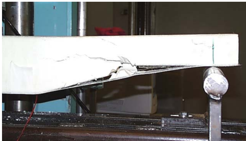
Figure 7.21 Failure of Neck Section #4
