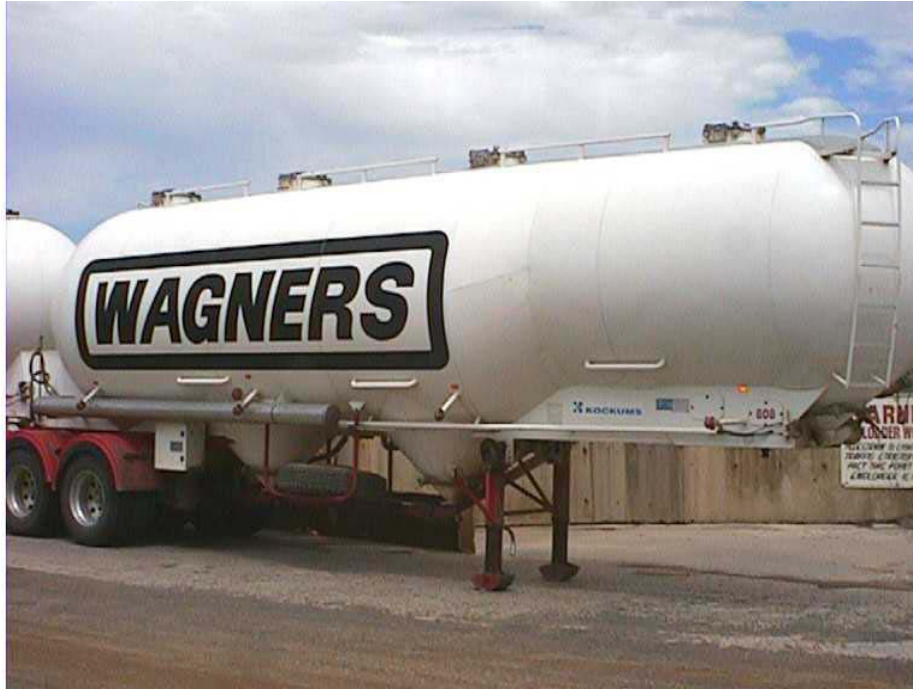
Figure 3.3 Tanker Used to Transport Cement Powder
