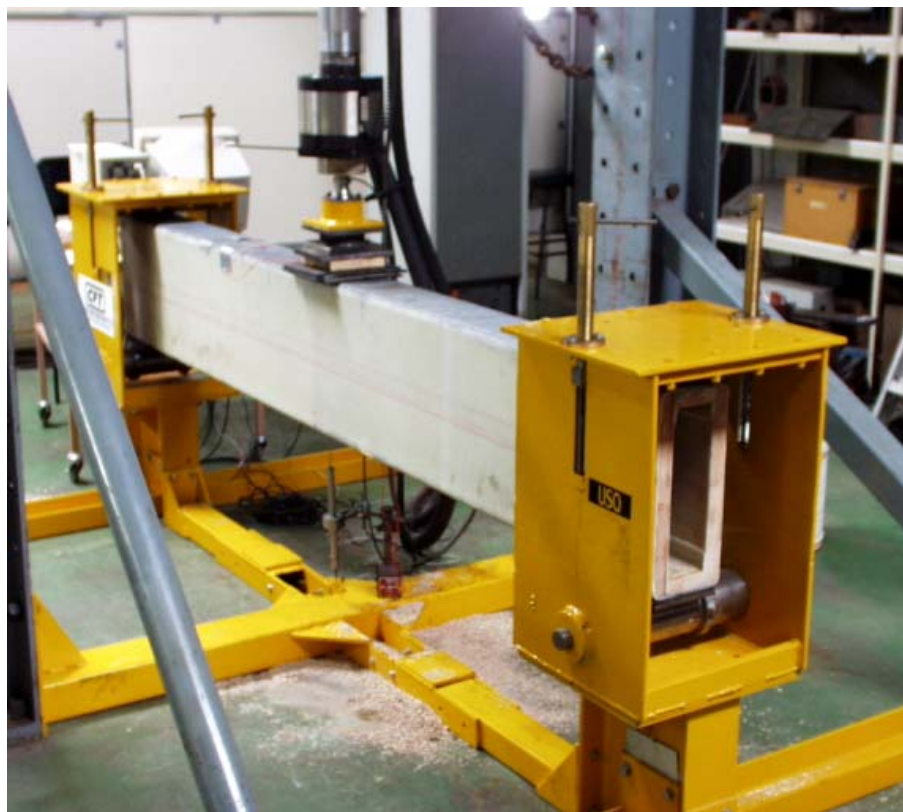
Figure G.15 Alternate View of Chassis Rail in Test Rig
