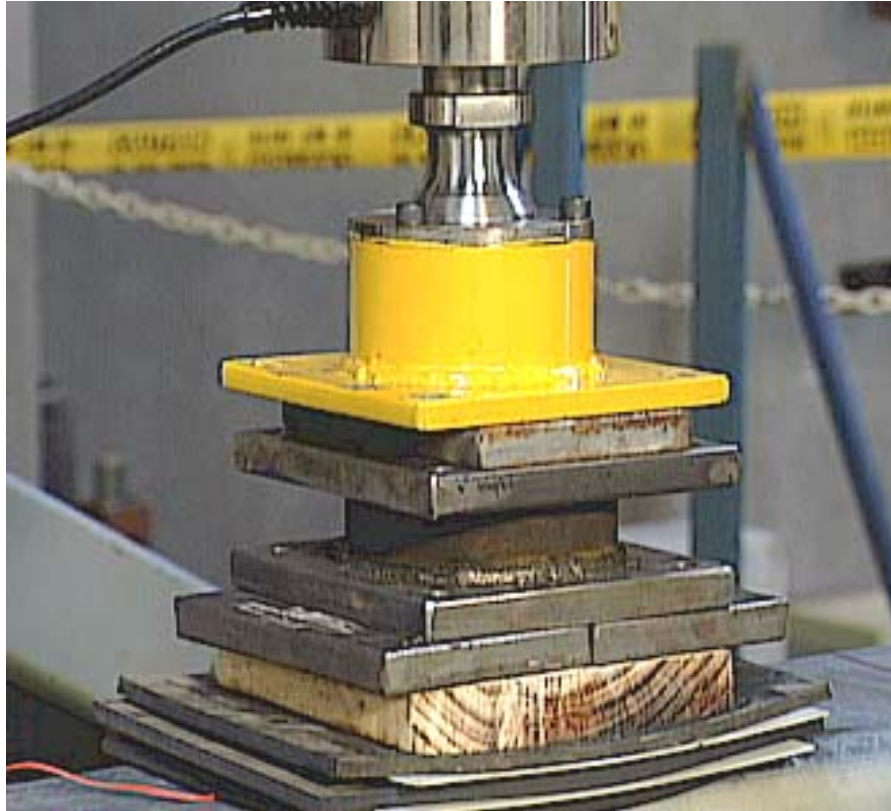
Figure G.16 Steel Spacers and Rubber Matting Used to Transfer and Distribute Load
