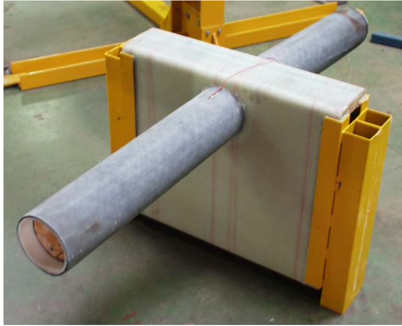
Figure F.6 Completed Test Piece Bonded to Steel Frame
