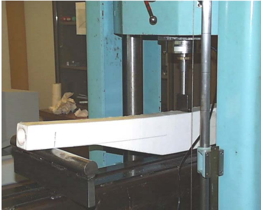
Figure D.12 (a) Neck Section #3 In Test Rig
