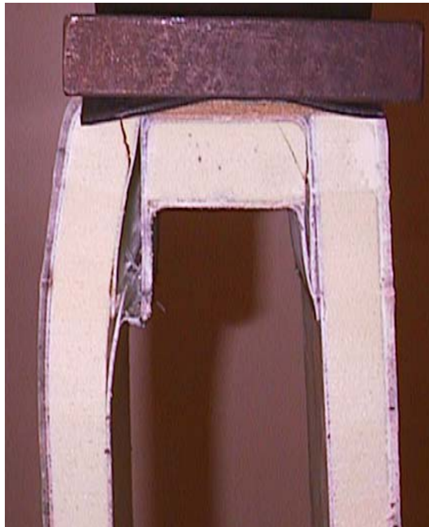
Figure C.11 (b) Ultimate Cross Sectional Failure through Delamination
