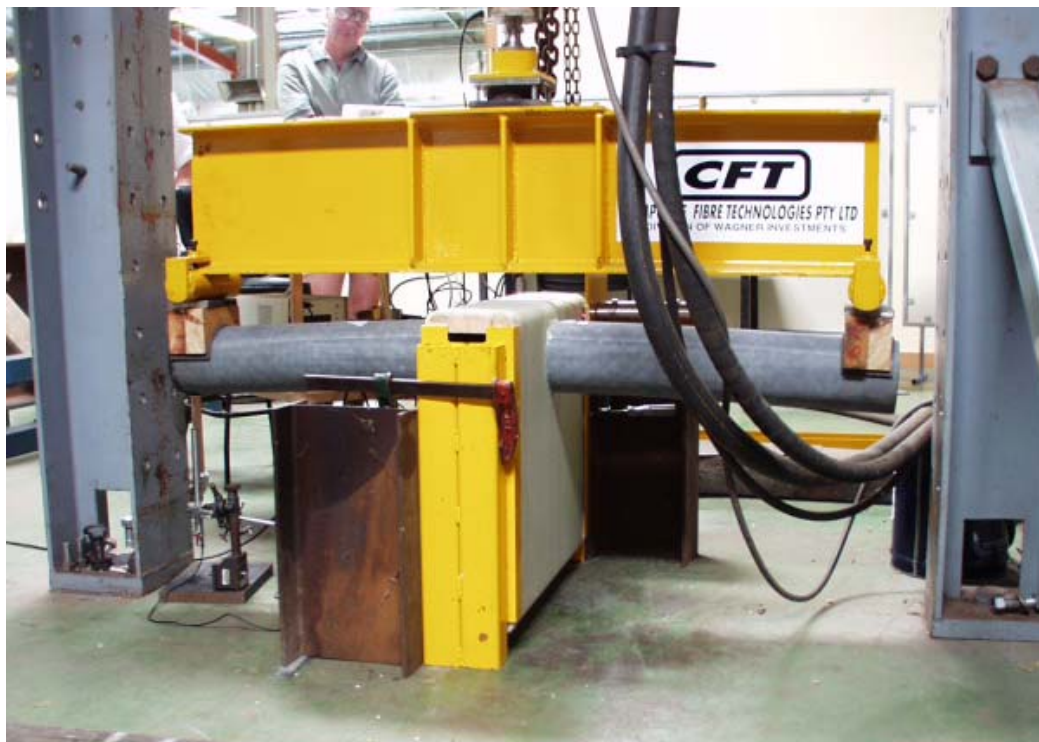
Figure F.9 Flexure of Cross Member during Testing
