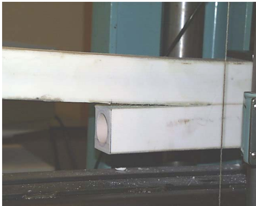
Figure D.11 (b) Failure of Neck Section #1
