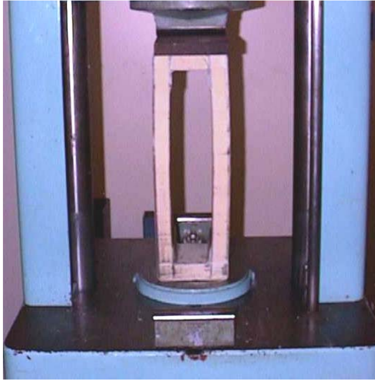
Figure C.11 (a) PU Section With First Core Crack (Top Right Side)
