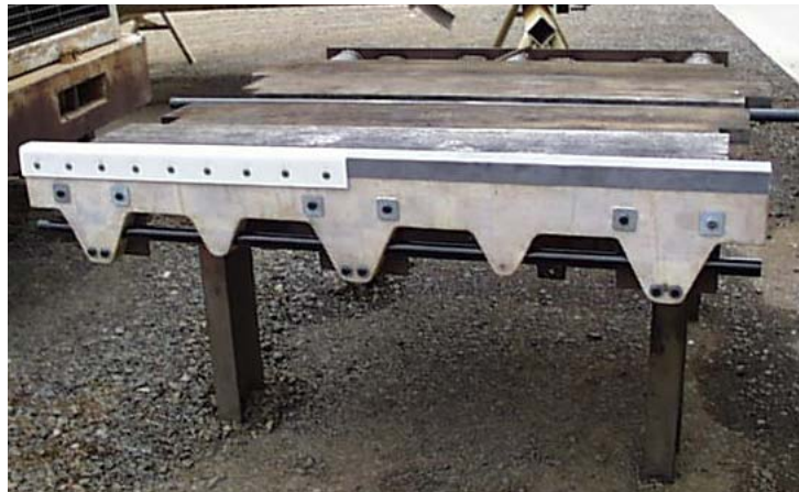
Figure 7.43 Prototype Combing Rail Prepared for Collision Test
