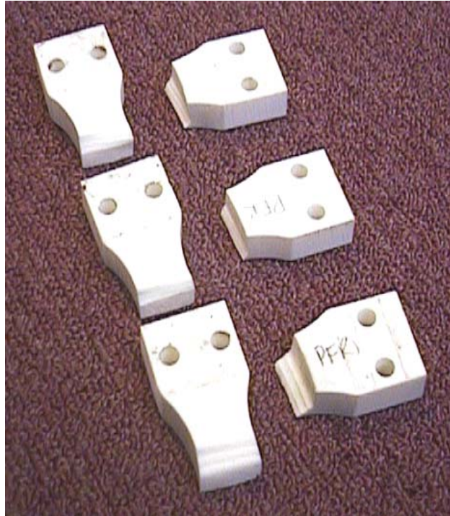
Figure G.3 Failure of Several PFR Fatigue Specimens
