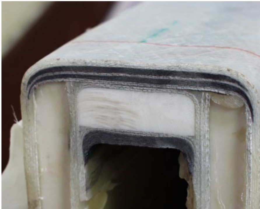
Figure E.10 Completed Beam Showing Laminate Wrap Sequence
