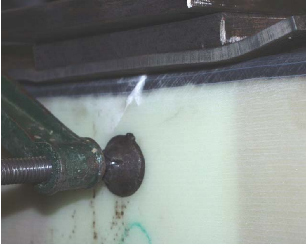
Figure E.11 (c) Initial Failure Point Beneath Load Pad
