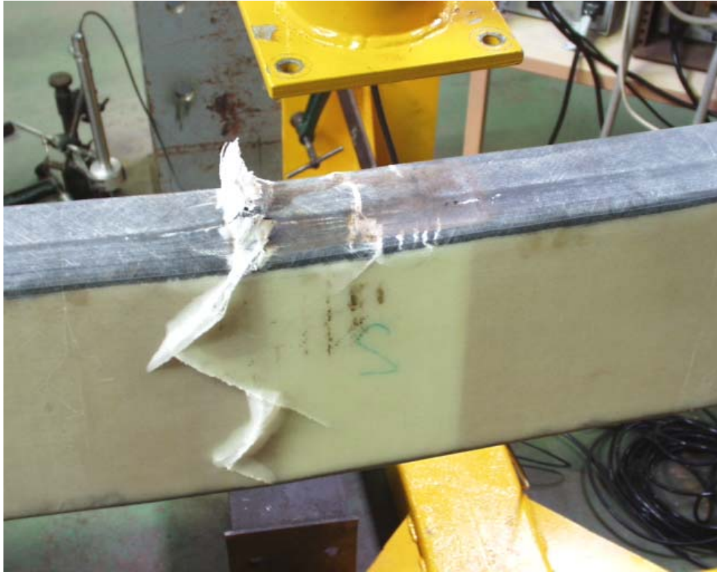
Figure E.11 (e) Both Failure Points with Load Pad Removed
