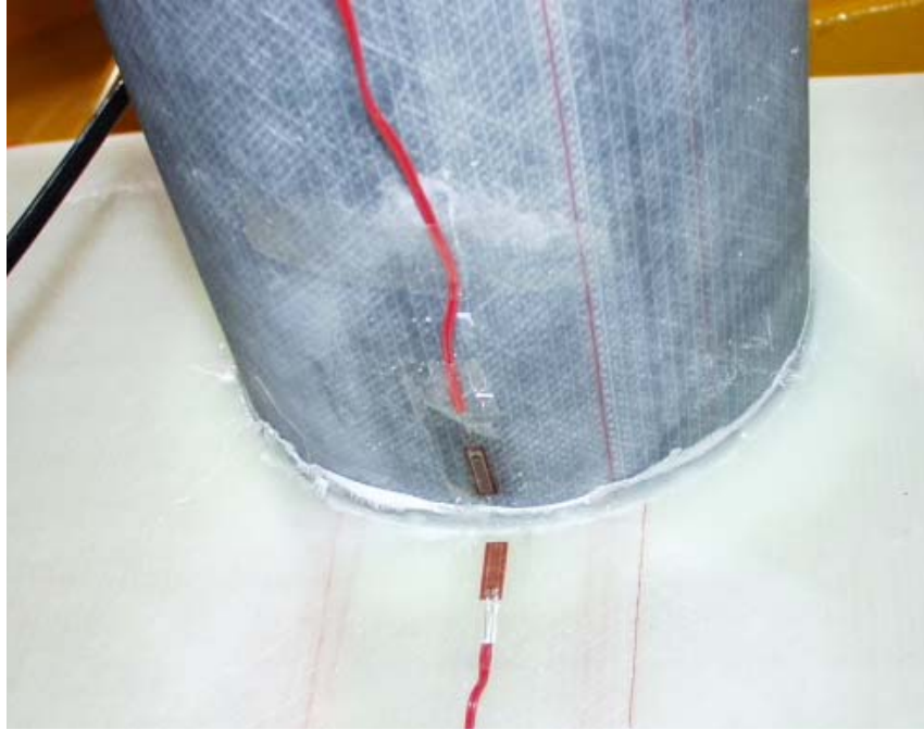
Figure F.7 (a) Strain Gauges Two and Three Placed on Underside of Cross Member
