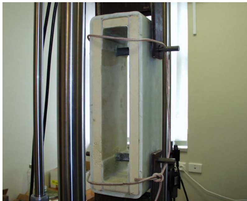
Figure 7.42 Dynamic Test of Bolt Through Chassis Rail
