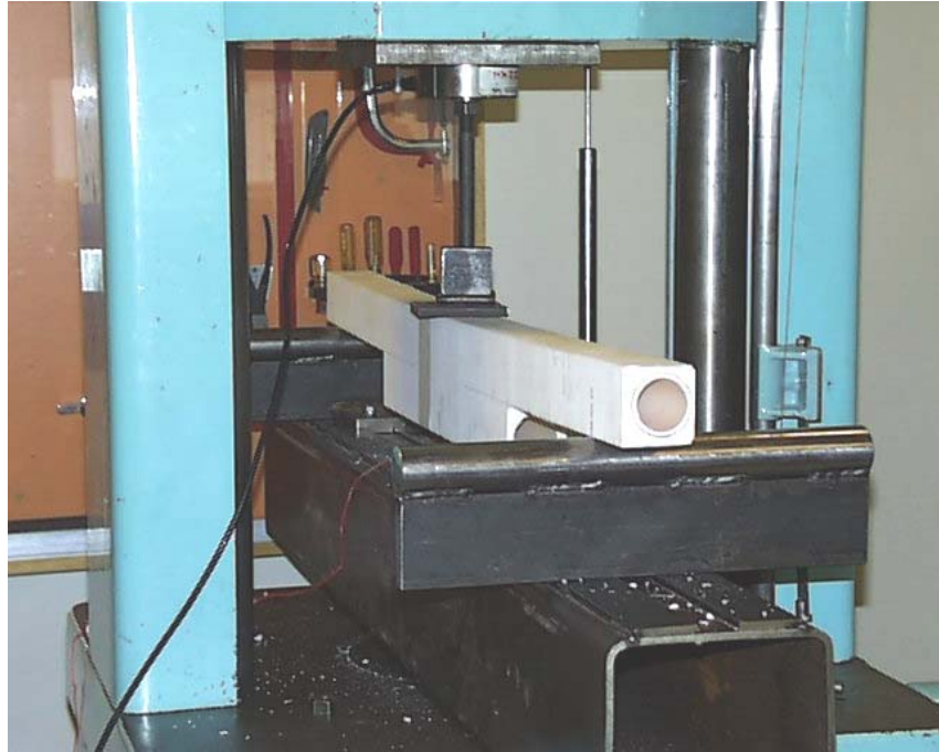
Figure D.11 (a) Neck Section #1 In Test Rig
