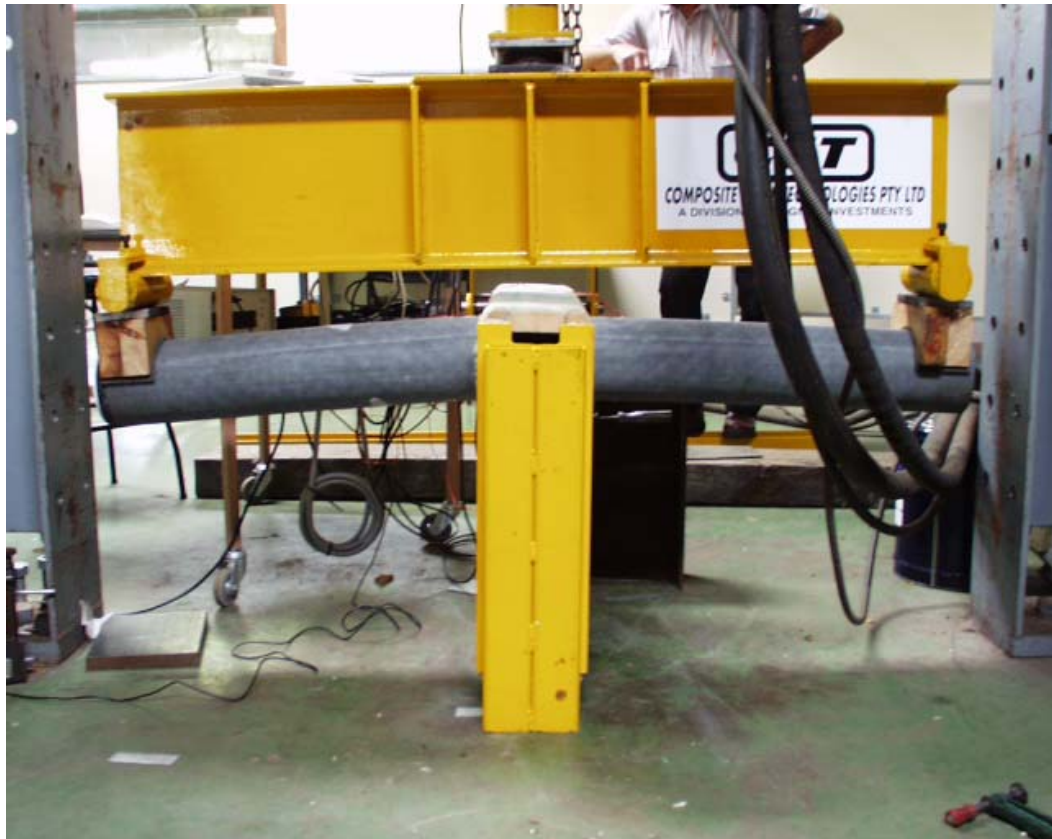
Figure F.10 Failure of Cross Member
