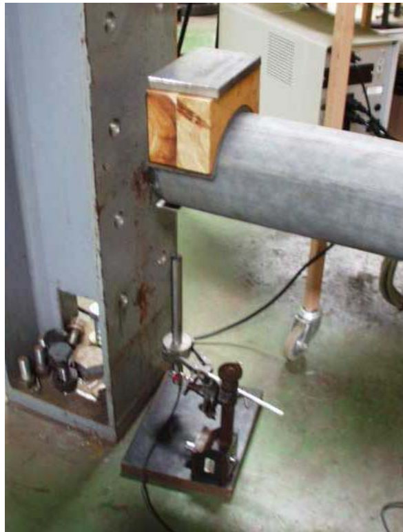
Figure F.8 Loading Platform and LVDT Placement
