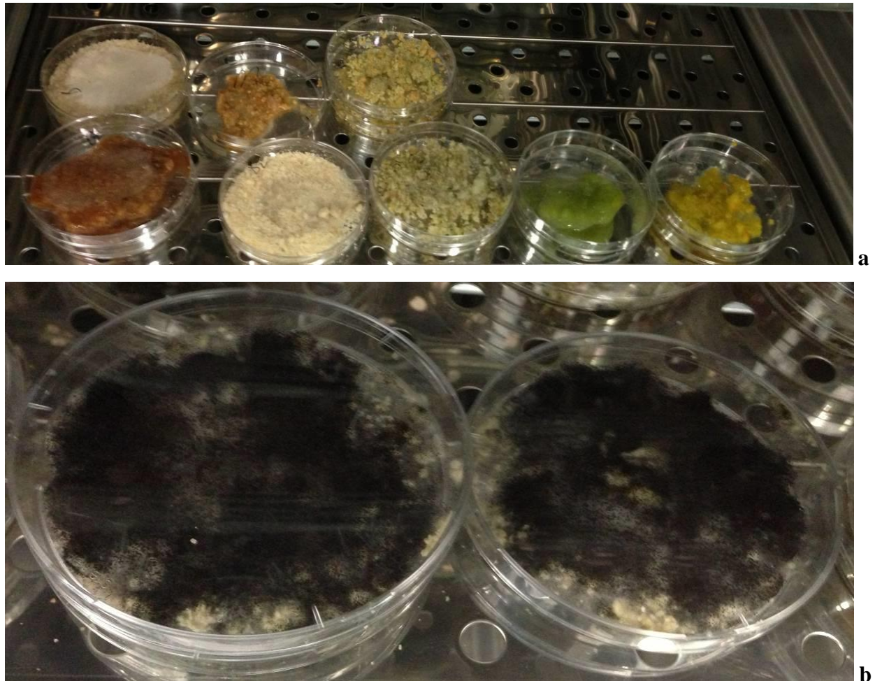
Figure 1. Solid state fermentation for enzyme production. a) Different FWs after fungal inoculation on day 0; b) Fungal micelles on cake wastes on day 4.
