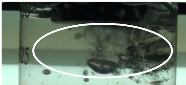
**Figure 4.9:** Generation of large air bubbles in the suspension with ultrasonic intensity of  $24.17 \text{ W/cm}^2$
