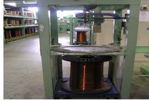
Figure 2: Existing wire mounting and tension setup
