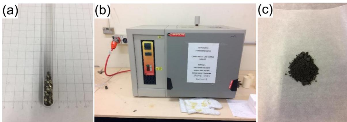
**Figure 3.2** Quartz tube and furnace for solid-solution synthesis. (a) Quartz tube with pre-weighted precursors inside. (b) Laboratory furnace used for solid solution synthesis. (c) As-ground  $\text{Bi}_{0.5}\text{Sb}_{1.5}\text{Te}_3$  powders.
