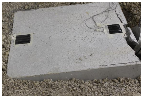
Figure 14. Vertical displacement of concrete floodway Specimen 2 at failure.
