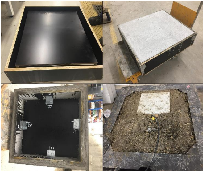
Figure 10. Formwork and casting concrete test specimen.
