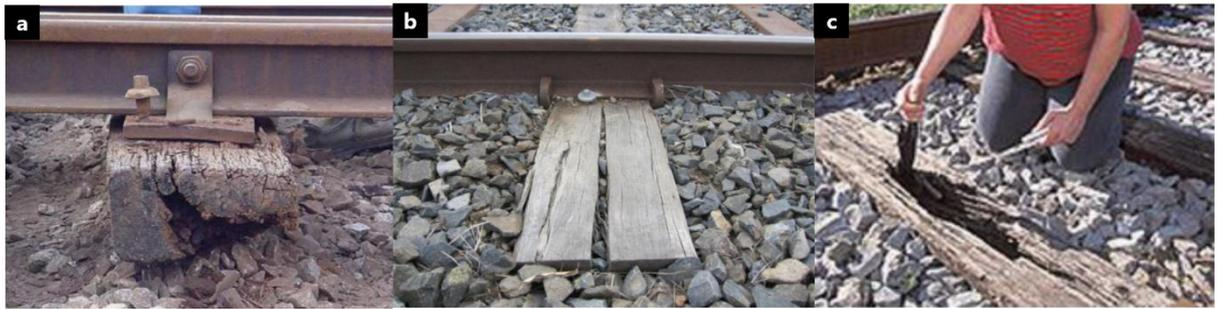
Figure 2: a) fungal decay (Manalo et al. 2010), b) end splitting, and c) termite attacks (Spillman 2003) in timber sleeper.
