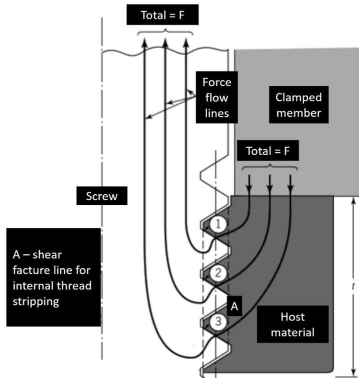
Figure 1: Force flow for a fastener in pull-out [43]
