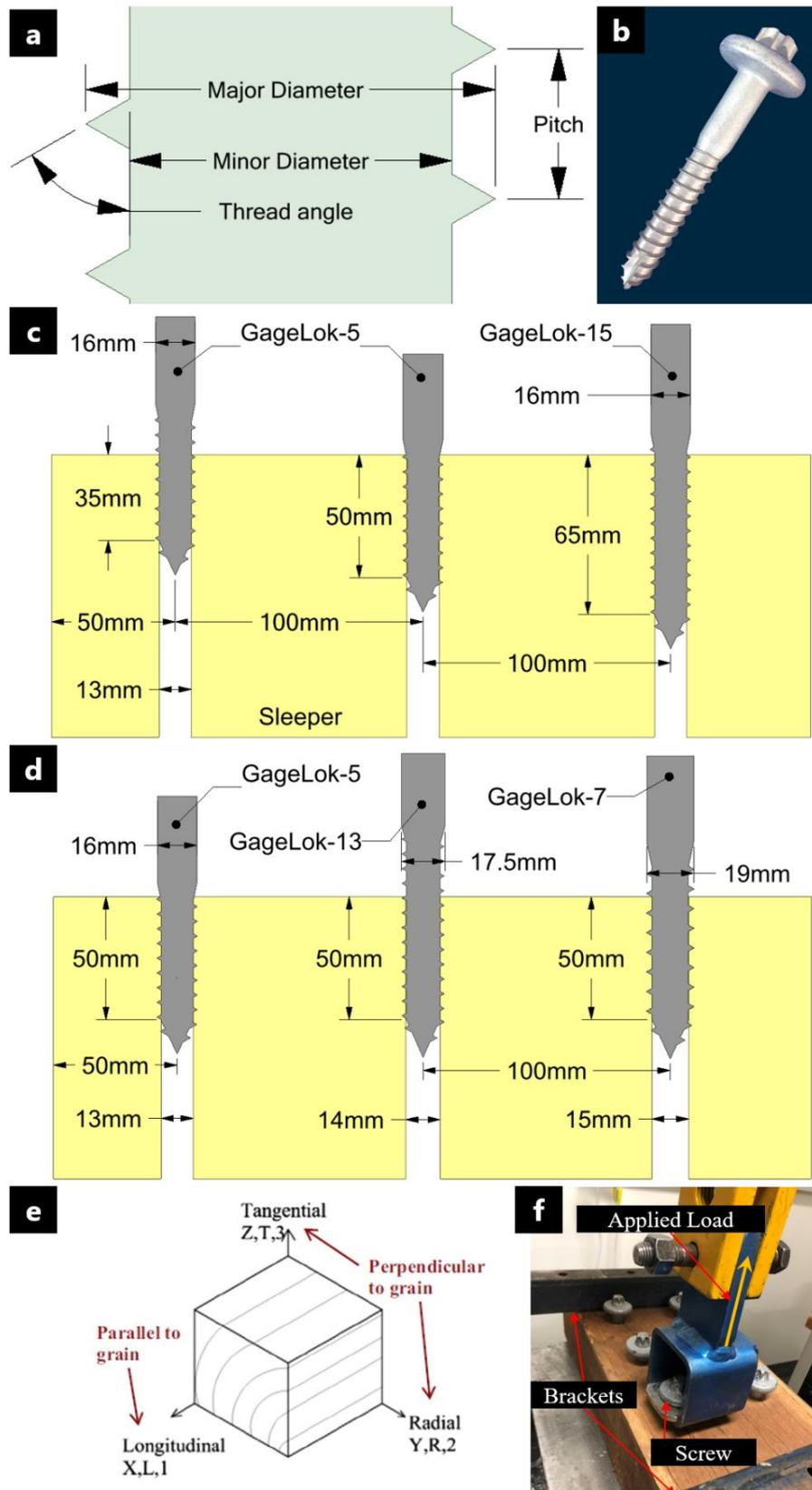
Figure 2. a) Terminology of the screw profile, b) the GageLok-11 rail screw, c) screw installation diagram with varied thread embedded length, and d) screw installation diagram with varied major diameter, e) definition of material directions of orthotropic material, f) screw pull-out test setup.
