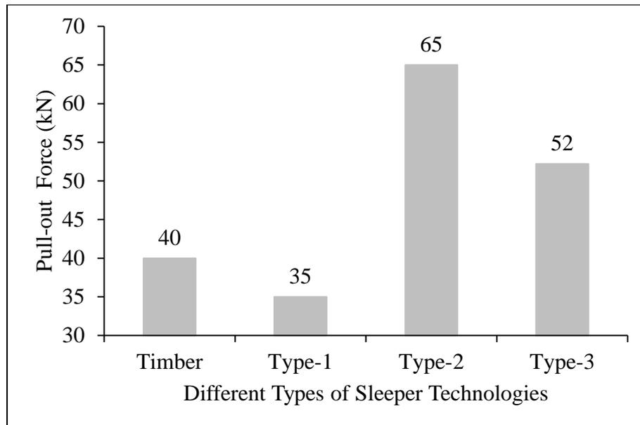
Figure 4: The screw pull-out performance of different types of sleepers (Ferdous et al. 2015)
