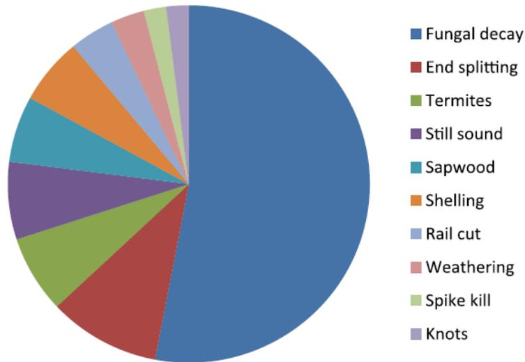
**Figure 1: Common causes of timber sleeper failure (Ferdous & Manalo 2014).**
