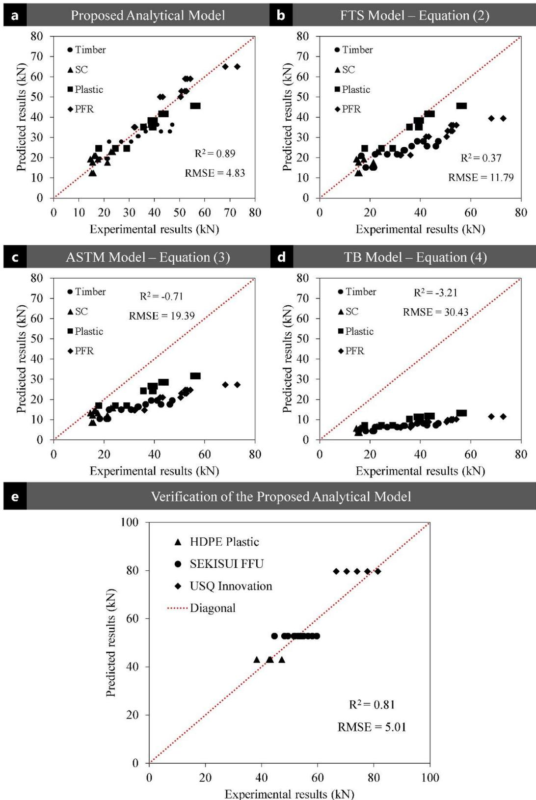
Figure 4: Comparison between the a) proposed model and b) - d) existing prediction models, e) verification with the data from literature
