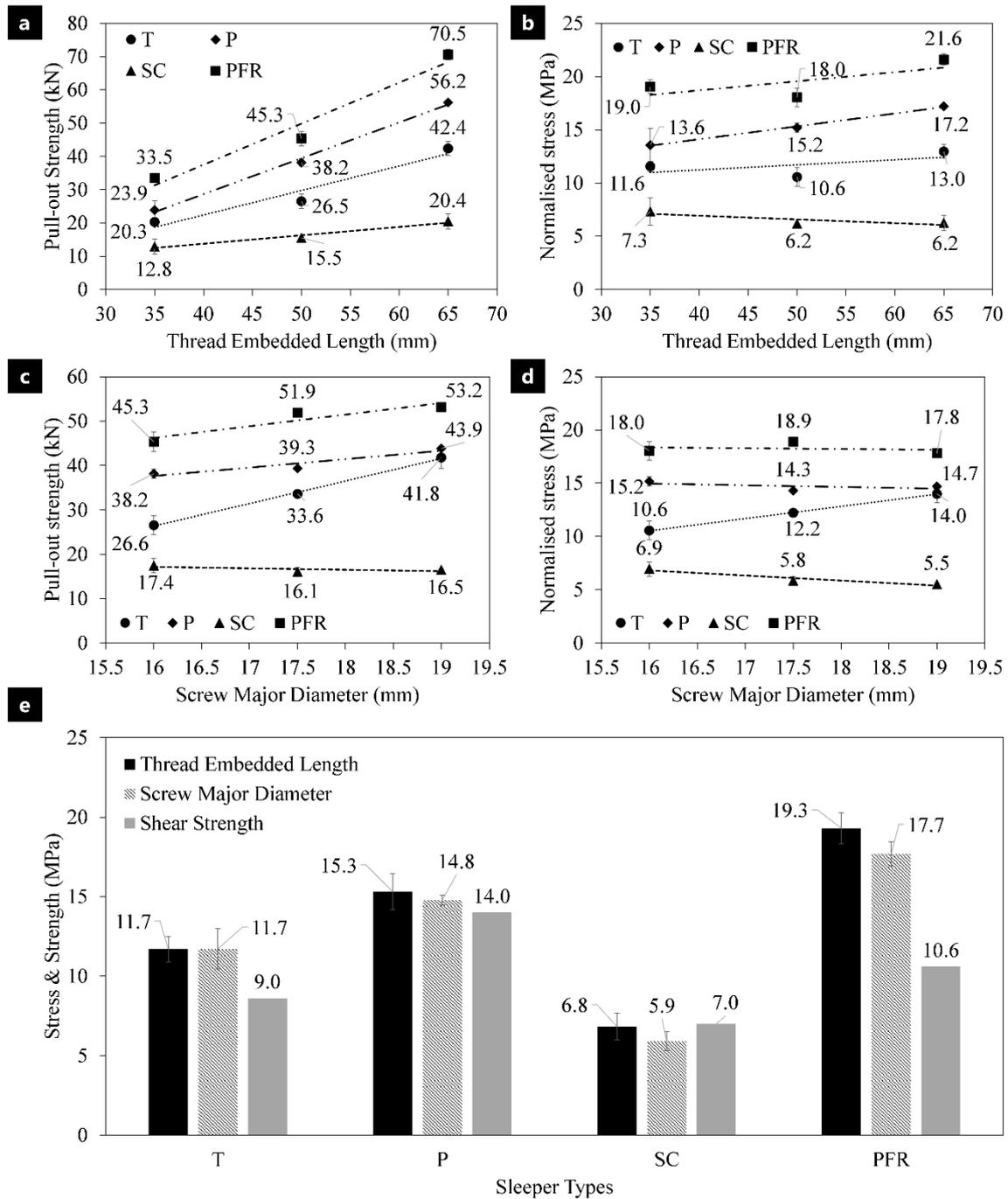
Figure 3: Increasing thread length (mm) plotted against a) pull-out strength (kN) and b) normalised stress (MPa); increasing screw major diameter (mm, discussed in Section 3.2) plotted against c) pull-out strength and d) normalised stress of timber (T), synthetic composites (SC), UHMWPE plastics (P), and PFR; e) average normalised stress compared to the sleepers' shear strength (MPa).
