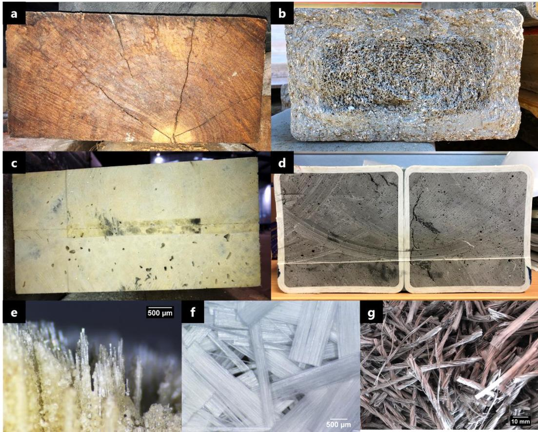
**Figure 3: Cross-section of railway sleepers, a) timber, b) recycled plastic, c) synthetic composite, and d) PFR core confined by laminates; adopted fibre reinforcement, e) long continuous glass fibre in the longitudinal direction of synthetic composites, f) short glass fibres or g) macro polypropylene fibres added to the PFR core (Yu et al. 2021).**
