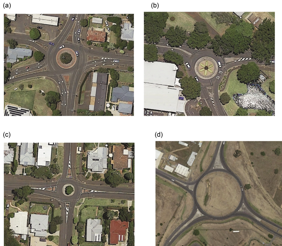
Fig. 3 – Examples of roundabout layouts (Google Earth, 2018). (a) 5-legged roundabout. (b) 3-legged roundabout. (c) First 4-legged roundabout. (d) Second 4-legged roundabout.
