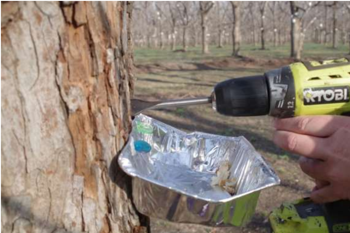
Figure 3.4: Sample collection, bark is being collected using a 25mm spade drill bit. Sample is collected in a foil tray
