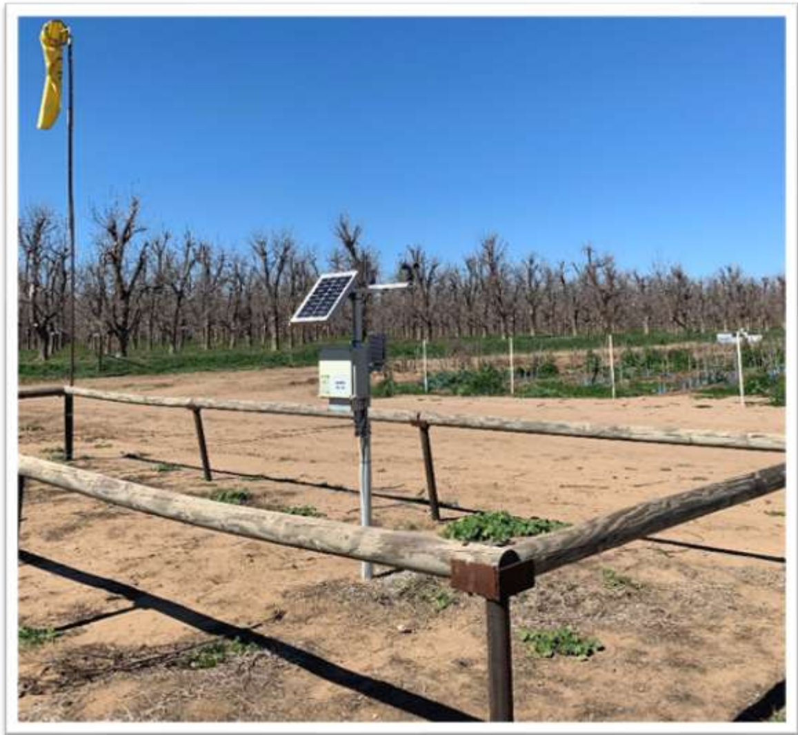
Figure 3.5: MEA weather station located at Trawalla airstrip measuring air temperature, solar radiation and rainfall.
