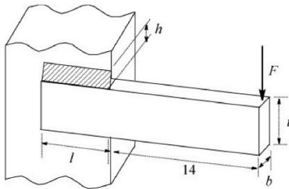
**FIGURE 5.** Problem of welded beam design.
