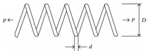
FIGURE 8. Tension/compression spring problem.
