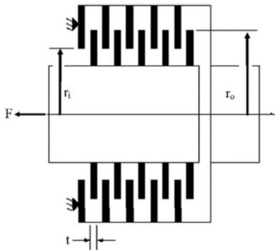
**FIGURE 10.** Multi-plate disc clutch brake problem.
