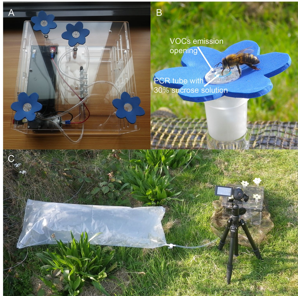
Fig. 1 Artificial flower setup: A general design, custom-made Perspex® box housing the volatile delivery system, B artificial flower, made of a glassware adapter with a Perspex® disk in the middle and flower petals made of foam sheets and C while in use in the field, covered with camouflage netting and attached bag filled with diesel exhaust
