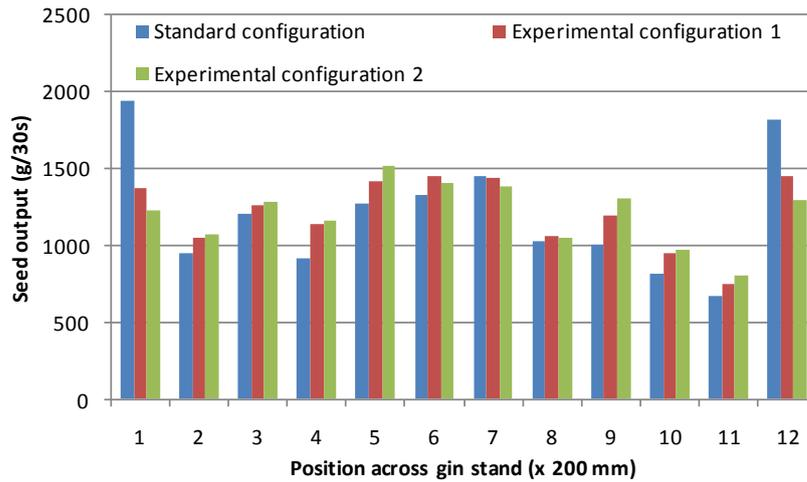
Figure 4-30: Seed cotton flow air manipulation – double pre-cleaner RH feed
