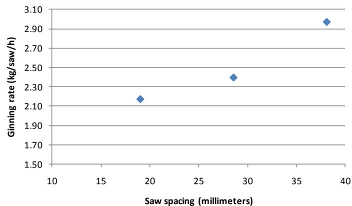
Figure 2-10: Ginning rate and saw blade spacing
