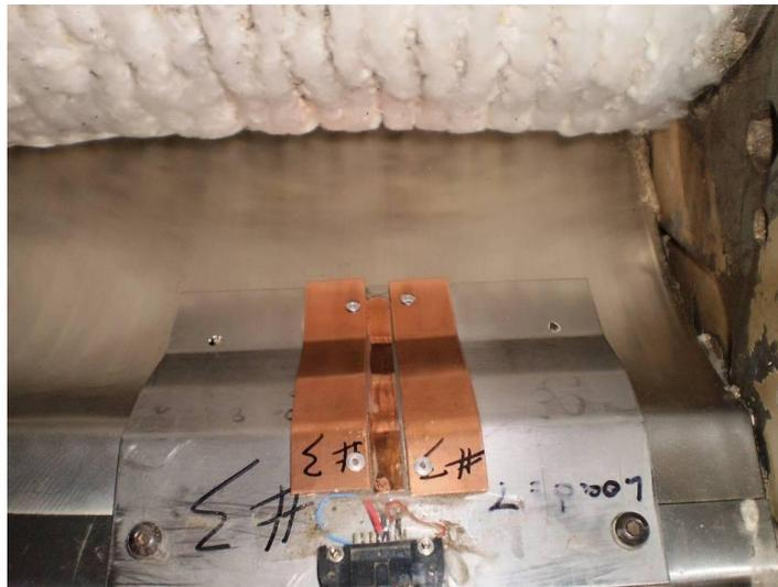
Figure 3-5: Seed roll force sensor positioned within roll box
