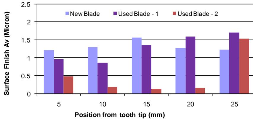
Figure 3-37: Saw blade surface finish (microns)
