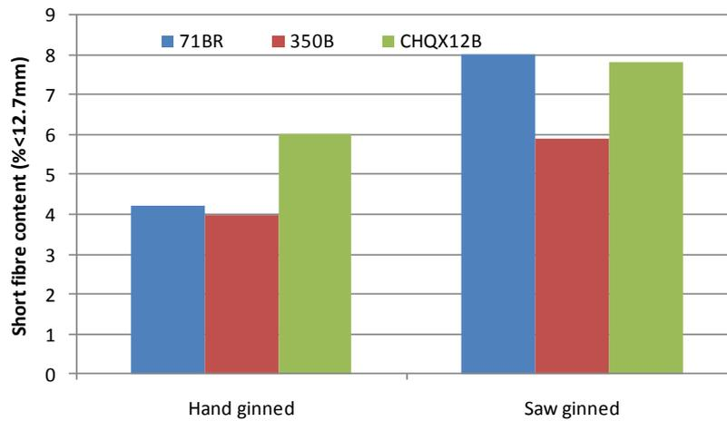
Figure 2-7: Hand ginning vs. saw ginning (SFC)
