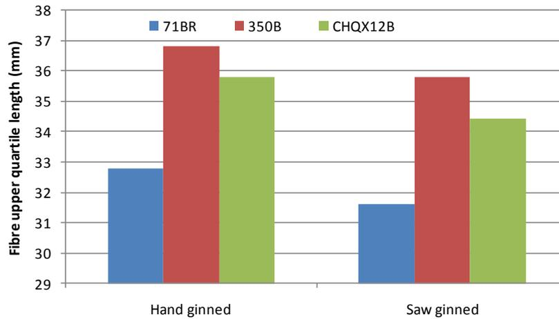
Figure 2-8: Hand ginning vs. saw ginning (UQL)
