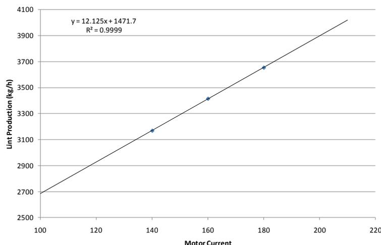
Figure 3-1: Motor current and lint production conversion chart
