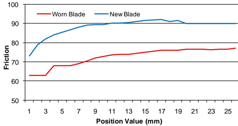
Figure 3-35: Saw blade surface friction – sample 2
