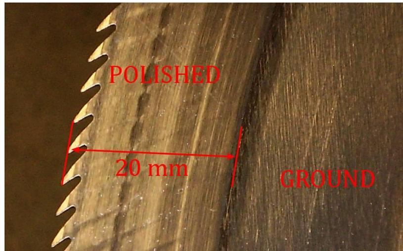
Figure 3-36: Saw blade surface finish
