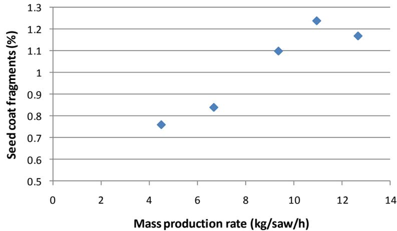
Figure 2-4: Seed coat fragments and ginning rate
