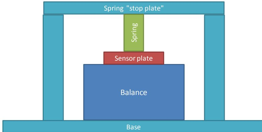
Figure 3-4: Force sensor calibration schematic
