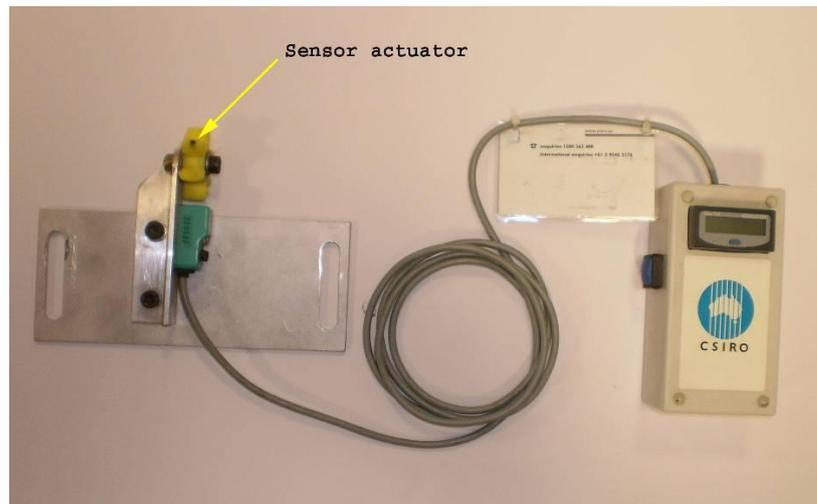
Figure 3-2: Seed roll tachometer
