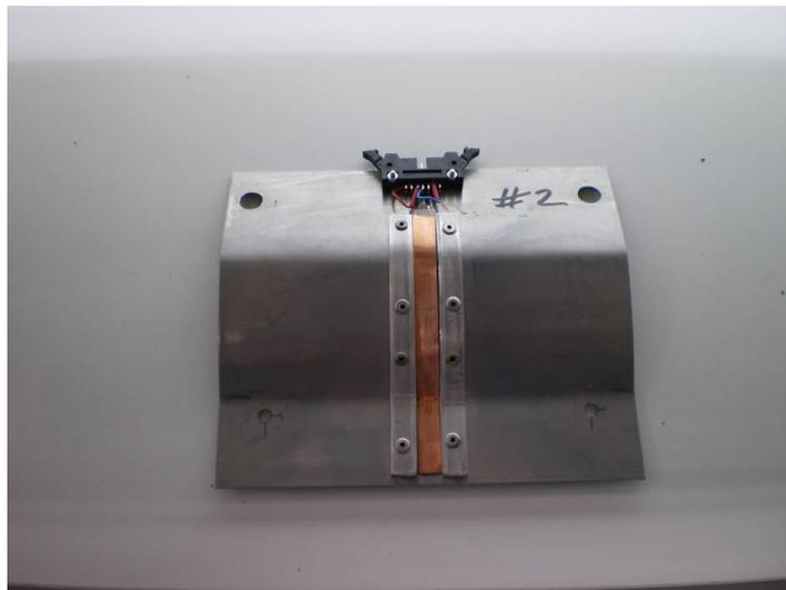
Figure 3-7: Seed roll force sensor Mk2
