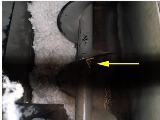
Figure 4-14: Conveyor distributor deflector mounted in position
