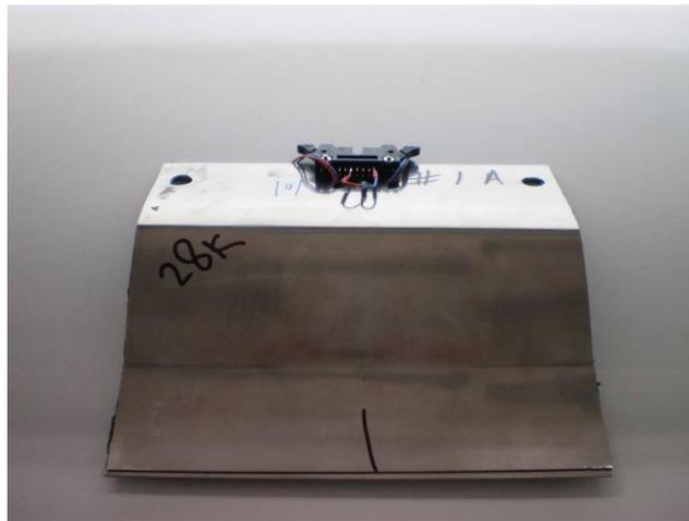
Figure 3-8: Seed roll force sensor Mk1
