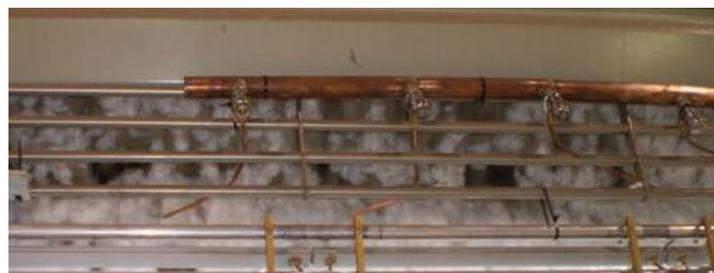
Figure 4-13: Air blowers in position to manipulate seed cotton distribution before the gin stand
