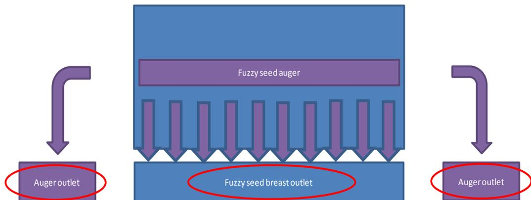
Figure 3-9: Fuzzy seed expulsion zones schematic
