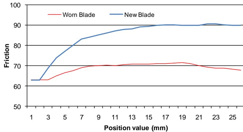
Figure 3-34: Saw blade surface friction – sample 1
