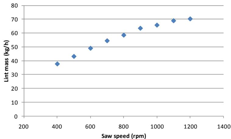
Figure 2-11: Ginning rate and saw shaft rpm
