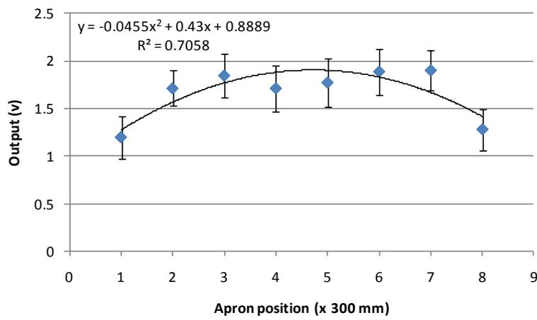
Figure 4-22: DAVS gin stand feed analyses–double pre-cleaner, RH seed cotton feed
