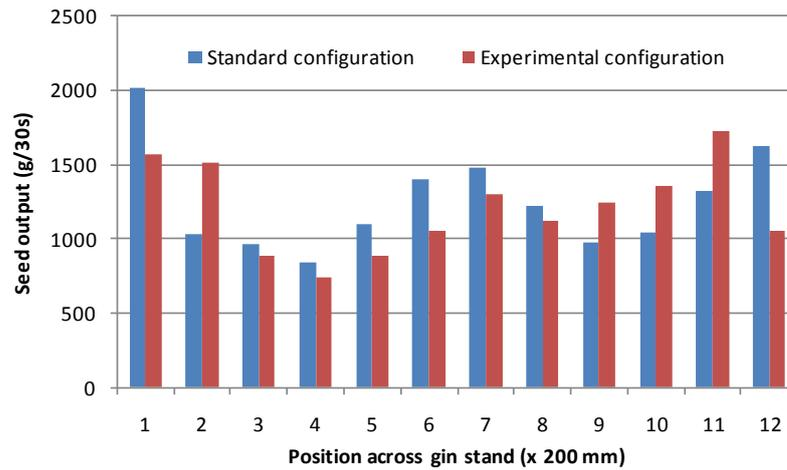
Figure 4-31: Gin stand conveyor distributor modification analyses
