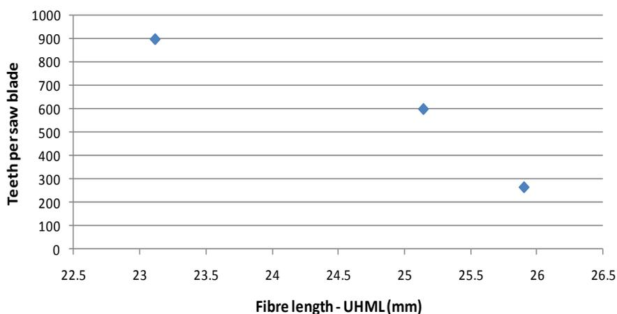
Figure 2-9: Saw blade teeth quantity/UHM
