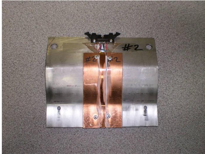
Figure 3-6: Seed roll force sensor Mk3
