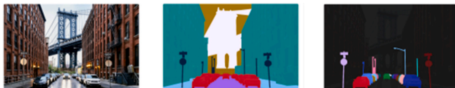
Fig. 13. Example of semantic and instance segmentation.
