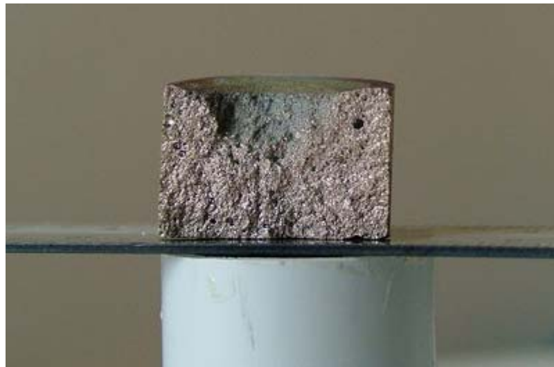
Figure 7: The specimen after being coated with a thin layer of gold
