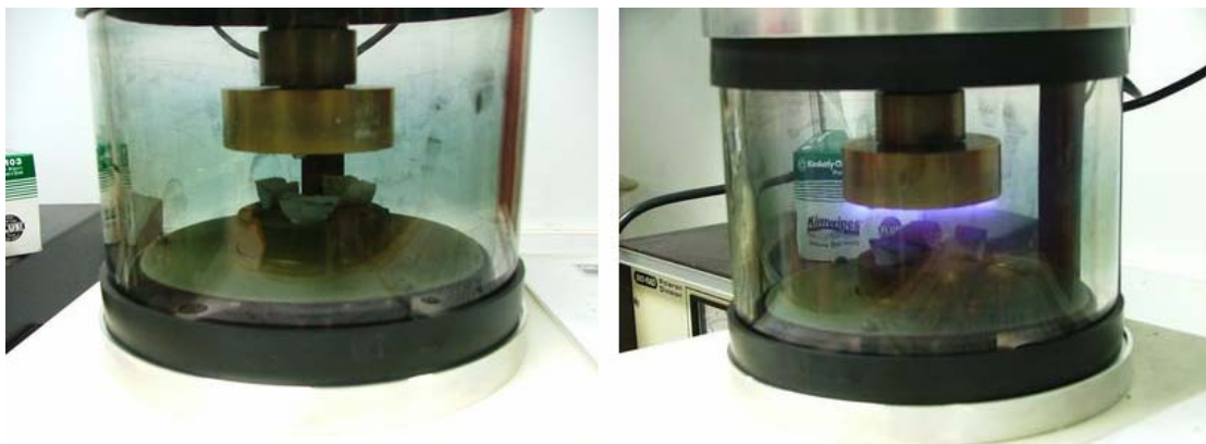
Figure 6: The sputter coater is coating a thin layer of gold on the specimen's surface
