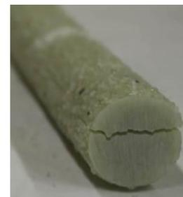
(c) Failure of #8 bars
