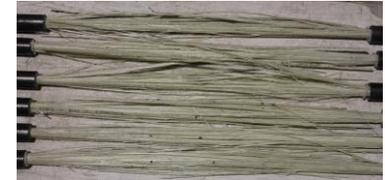
(c) Failure of #8 bars
