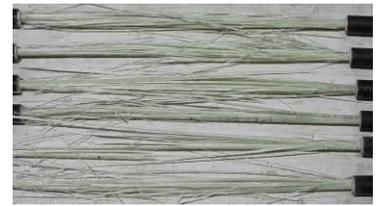
(b) Failure of #3 bars
