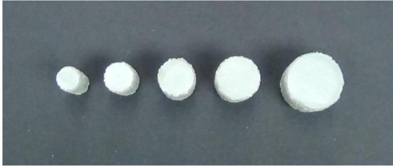
Figure 1 – Tested GFRP bars specimens
