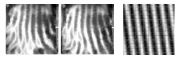
Figure 3. Oblique rolls for  $(Gr_m, Gr) = (15, 8)$ : "blinking" states observed experimentally (two left snapshots) and oblique waves obtained numerically (right).
