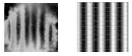
Figure 2. Magneto-convective instability: liquid crystal visualization (left) and the computed three-dimensional temperature field near the cold wall (right) for  $(Gr_m, Gr) = (10, 7)$ . Magnetic field is perpendicular to the plane of snapshots.
