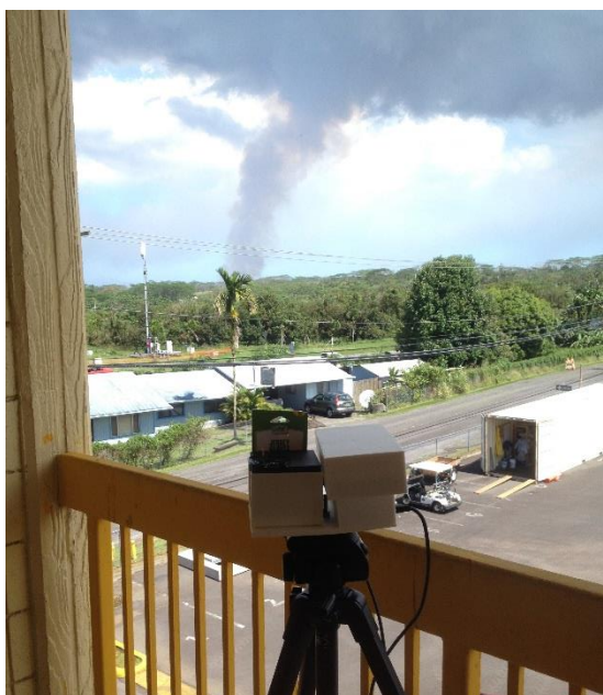
631 632 Figure 4- Raspberry Pi based spectrometer being used to measure gas release from fissure 8, Kilauea volcano, Hawaii – 633 August 2018. At this point in time, this vent was one of the most prodigious point sources on the planet of sulphur dioxide to 634 the atmosphere.
