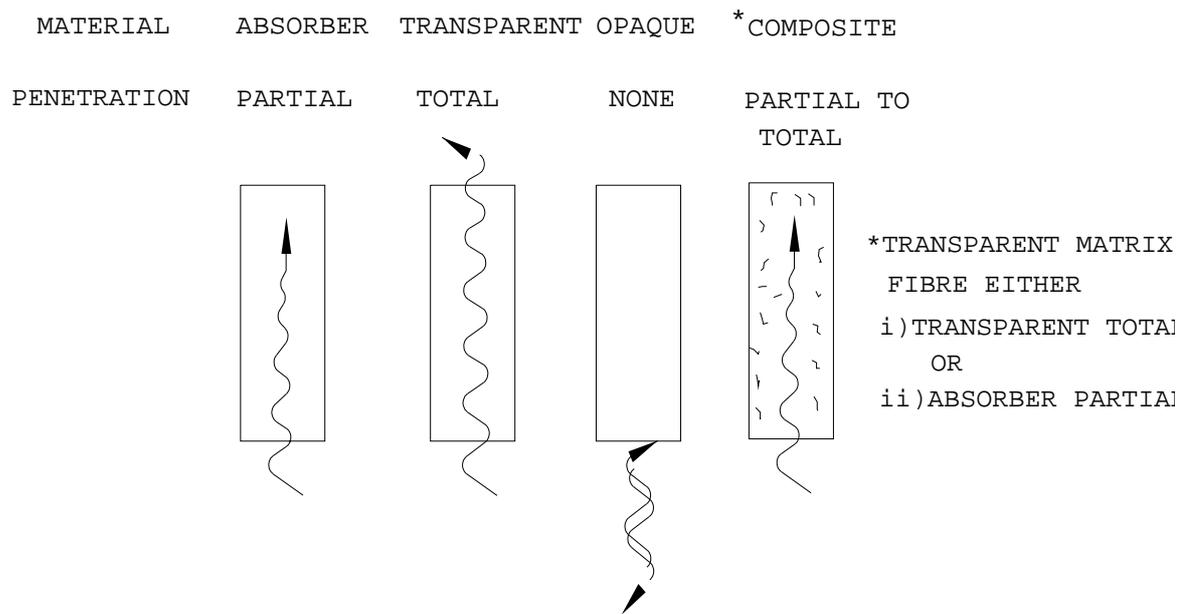
**Figure 7: Interaction of Microwaves with Materials**
