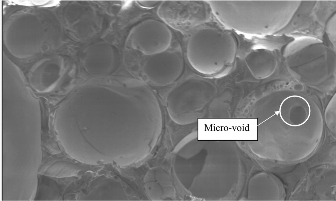
**Figure 16: The micro-void (bubble) is less in the composite cured under 180-watt and 60-second microwave irradiation.**
