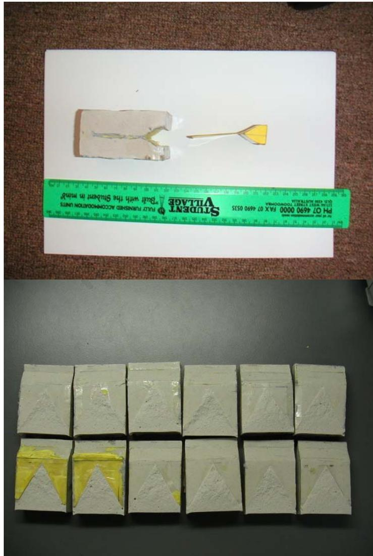
Figure 6: The short bar specimens
