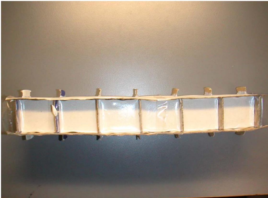
Figure 5: The mould for short bar specimens
