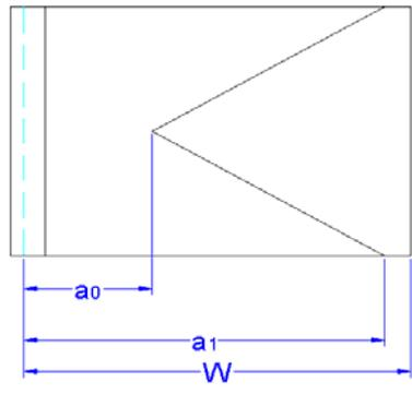
**Figure 14: Cross-section dimension of short bar specimen showing  $a_1$**
