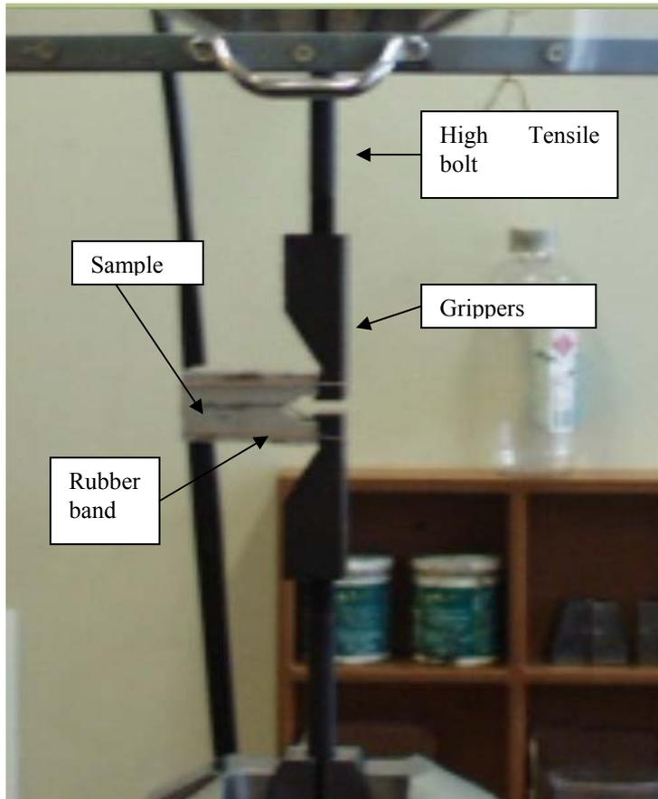
**Figure 10: Test rig with specimen in position.**
