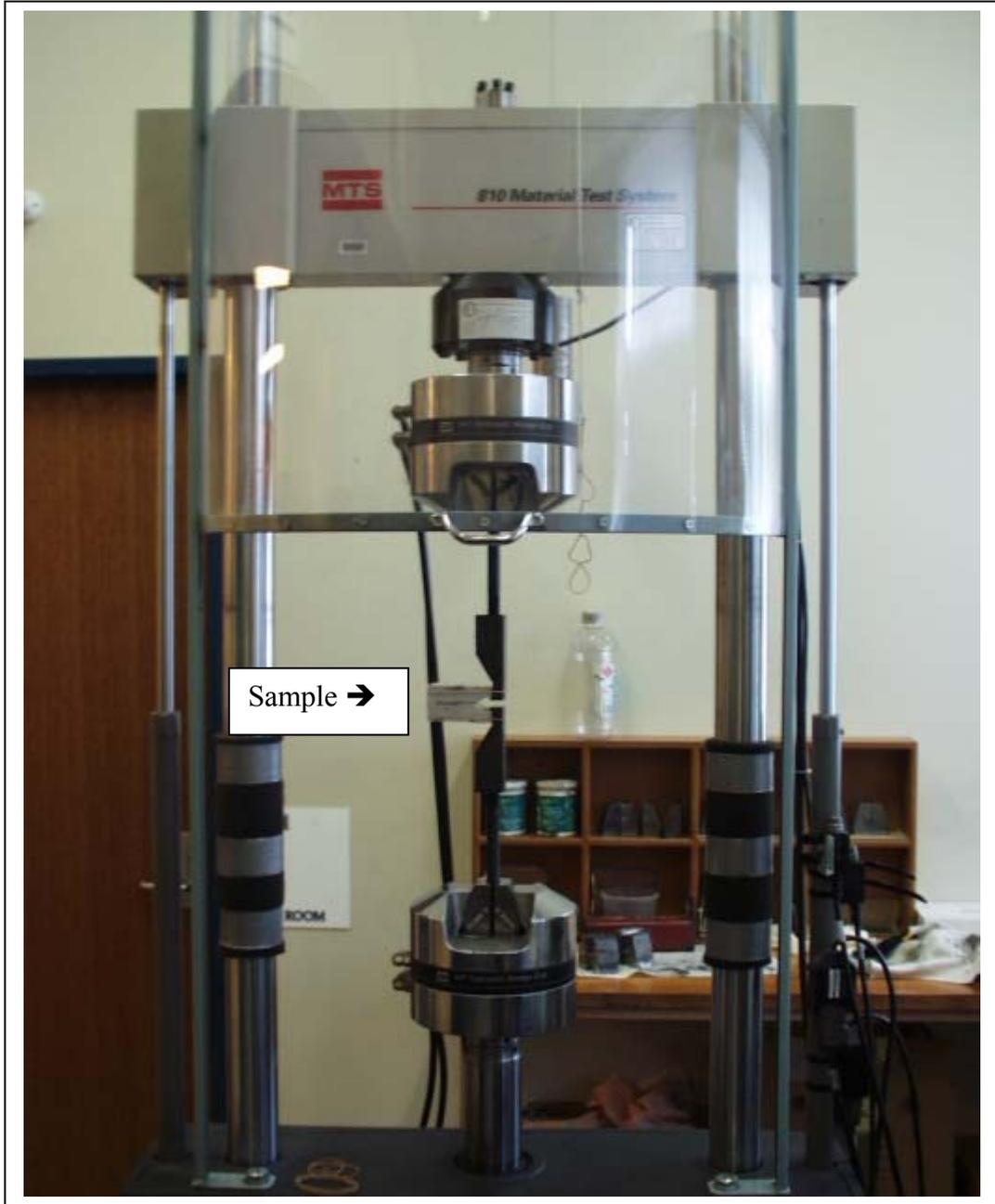
Figure 9: Fracture toughness test in process
