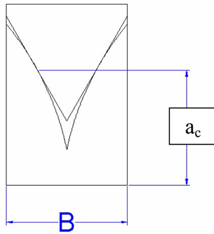
Figure 4: Curved and Straight Slots Tangent at  $a_c = 0.85B$ , in the short rod specimen geometries
