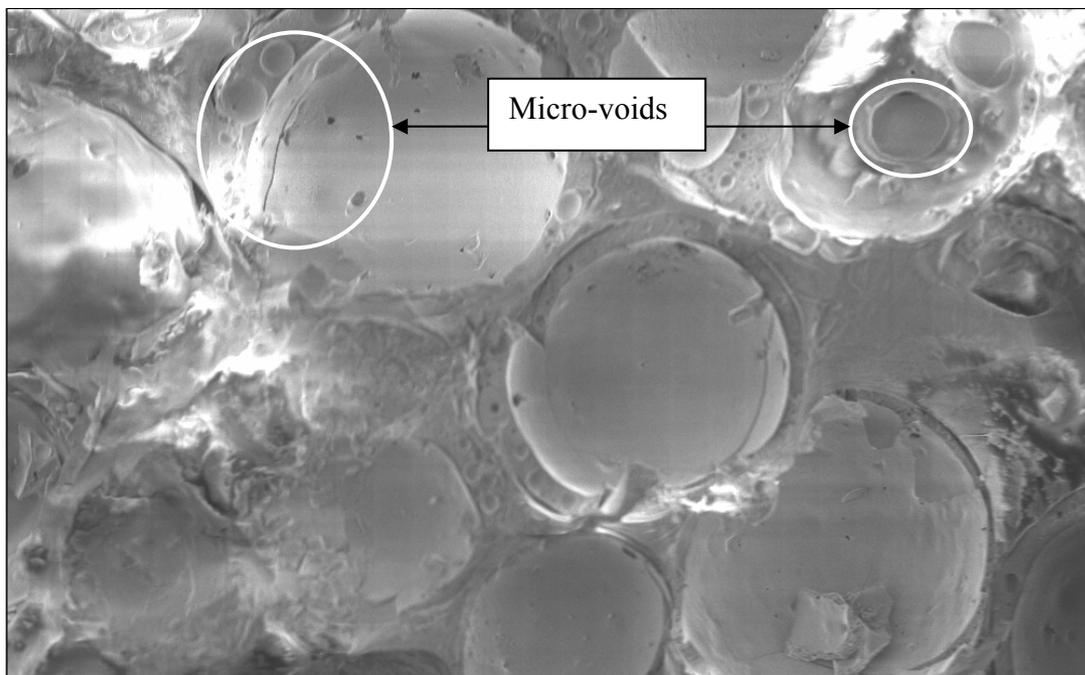
**Figure 15: Some micro-voids (bubbles) existed in the composite cured under 360-watt and 80-second microwave irradiation.**
