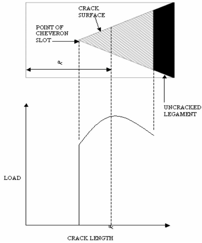
Figure 11: Variation of load versus crack length
