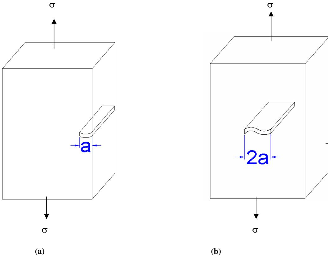
**Figure 1: Schematic Drawing of Fracture Toughness Specimens with Edge and Internal Flaws**
