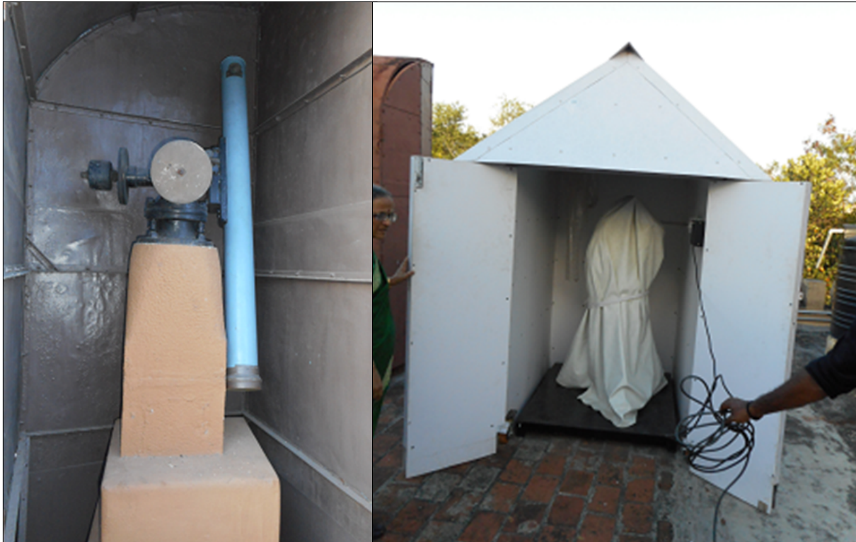
Figure 6: Left: a recent photograph of the historic equatorially-mounted 5-inch refractor at Trivandrum Observatory used by Professor Iyer to track Comet C/1941 B2 (de Kock-Paraskevopoulos) in January 1941. Right: The mobile 'observatory' in which the telescope currently is housed when not in use on public viewing nights (photographs courtesy: Pramod Galgali).
