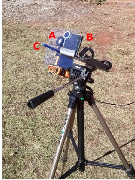
Figure 1: In situ image of the data gathering equipment for a sample sun-normal measurement. Both the smartphone camera (B) and the UVA sensor (A) are arranged beneath the 2 mm clear glass sample slide. The sun targeting apparatus protrudes from the front of the array (C).
