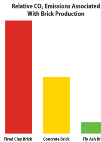
Figure 4.10: CO 2 emissions of different brick types Source: Volz and Stovner (2010); Structure Magazine (2014);
